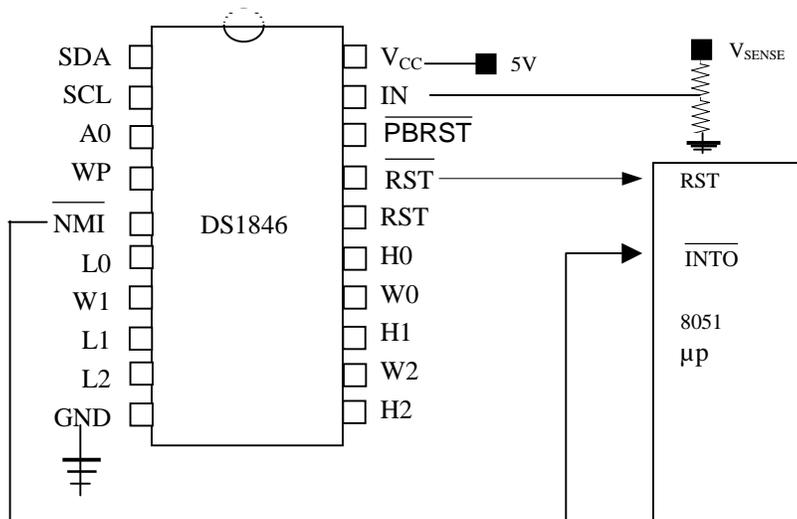
$$V_{\text{SENSE}} = \frac{R1 + R2}{R2} \times 1.25$$
