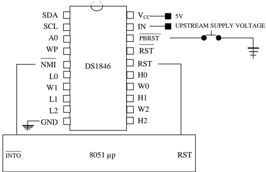
**PUSHBUTTON RESET CONTROLLED BY NMI Figure 5**
