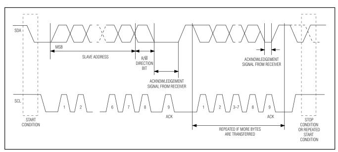
Figure 2. 2-Wire Data Transfer Protocol
