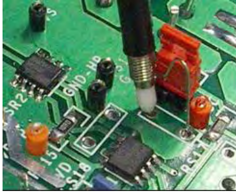
Fig. 4A Direct gate voltage probing using tip & gnd spring.
