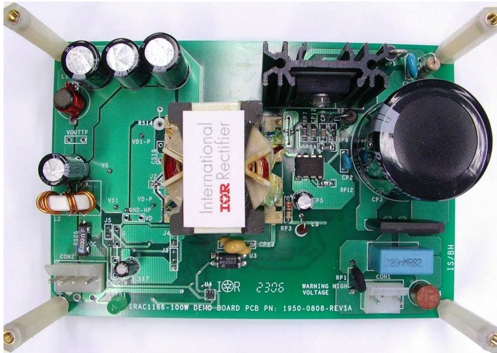
Figure 2A. Top side of the IRAC11662-100W Demo Board
