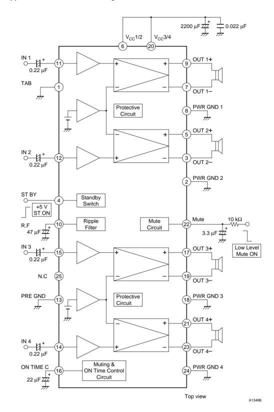
Sample Application Circuit and Block Diagram
