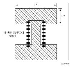
FIGURE 2. Copper Heatsink Patterns
