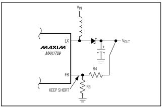
Figure 4. Adjustable Output Voltage
