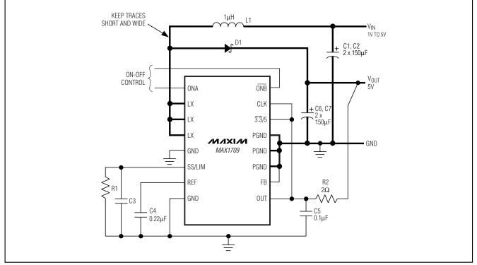
Figure 1. Standard Operating Circuit
