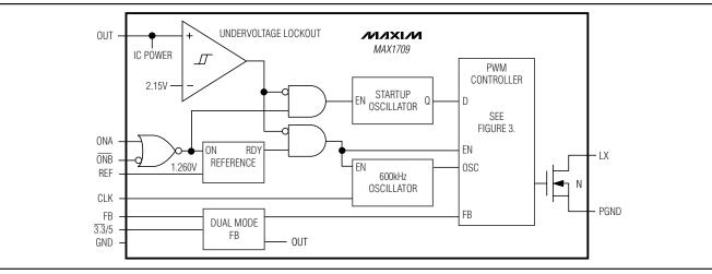
Figure 2. Simplified Functional Diagram
