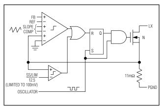
Figure 3. Simplified PWM Controller Functional Diagram
