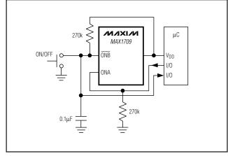
Figure 5. Momentary Pushbutton On-Off Switch
