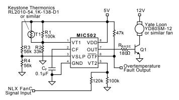
Figure 7. Typical 5V V<sub>DD</sub> Application Circuit
