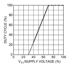
Figure 6. Control Voltage vs. Fan Speed
