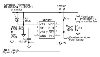
Figure 8. Typical 12V V<sub>DD</sub> Application Circuit
