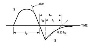
Figure 15. Diode Reverse Recovery Waveform
