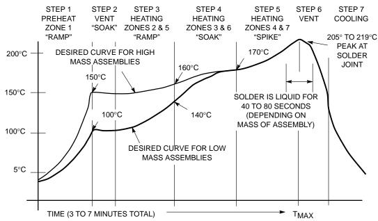
Figure 18. Typical Solder Heating Profile
