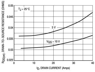
Figure 3. On–Resistance versus Drain Current and Temperature
