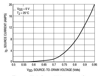
Figure 10. Diode Forward Voltage versus Current
