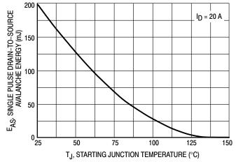
Figure 13. Maximum Avalanche Energy versus Starting Junction Temperature
