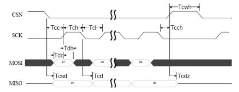
Figure 7 SPI NOP timing diagram
