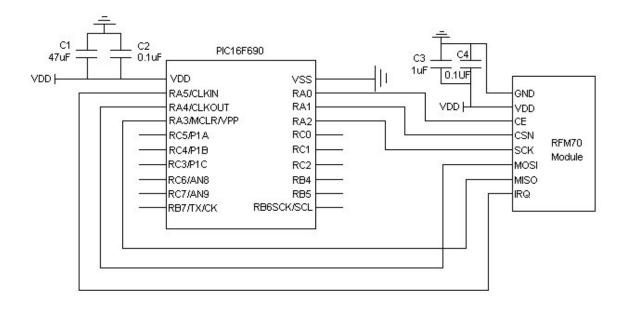
Figure 8 RFM70 typical application schematic
