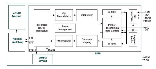
Figure 1 RFM70 Chip Block Diagram
