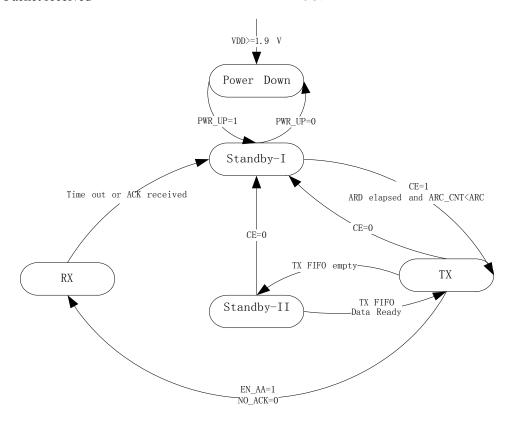
Figure 3 PTX (PRIM\_RX=0) state control diagram
