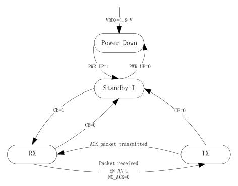
Figure 4 PRX (PRIM\_RX=1) state control diagram
