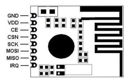
Figure 2 RFM70 pin assignments (top view)
