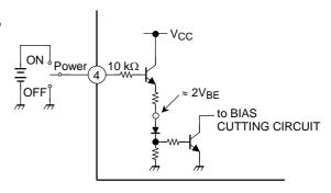
Figure 2 With pin 4 set to High, Power is turned ON
