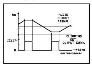
takes the form of pulses, which are perfectly syncronized with each single clipping event in the music program and reflect the same duration time (fig. 5). Applications making use of this facility usually operate a filtering/integration of the pulses train through passive R-C networks and realize a volume (or tone bass) stepping down in association with microprocessor-driven audioprocessors.
