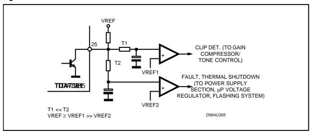
tor has to be viewed mainly as a power-dependent feature rather than frequency-dependent. This means that clipping state will be immediately signaled out whenever a fixed power level is reached, regardless of the audio frequency.
