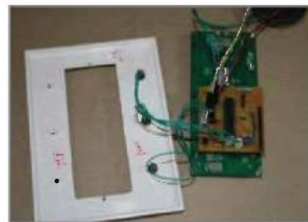
Photo 3 —The microcontroller board is attached to the LCD module with its push buttons attached to a wall plate. I used a nibbling tool to cut out the LCD viewport. After the bezel was installed, the appearance dramatically improved.
