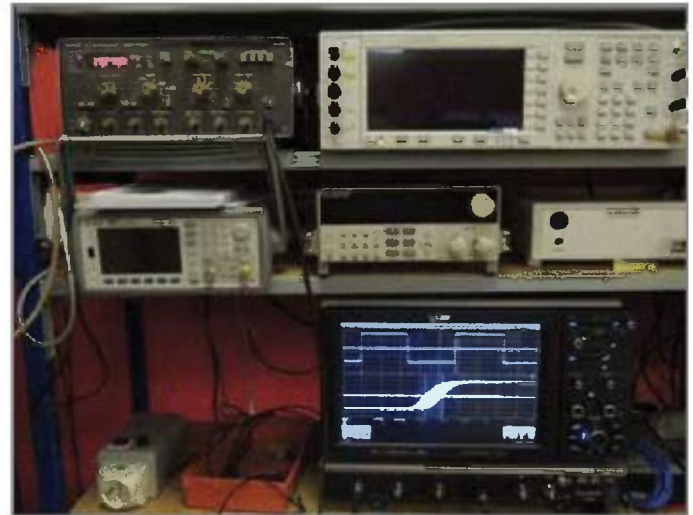
Photo 1— Here is the test setup. The partially faulty PM5134 generator is on the top left. The LeCroy WaveRunner oscilloscope, which shows a high level of jitter, is on the bottom.
