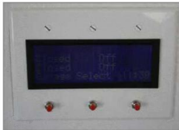
Photo 1 —The completed control panel includes a three-gang wall box. I used a nibbling tool to cut out the display's bezel.
