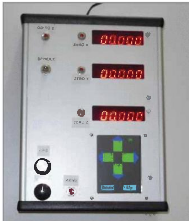
Photo 1 —Atmel's ATmega88 and ATmega1284 microcontrollers are at the heart of the CNC controller.
