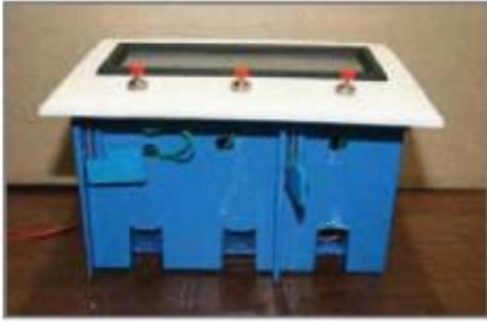
Photo 4 —The unit is assembled and inserted into a three-gang wall box, ready for mounting. There are three screws holding the faceplate on the top and the push buttons are screwed to the faceplate and slid into the wall box's screw holes.
