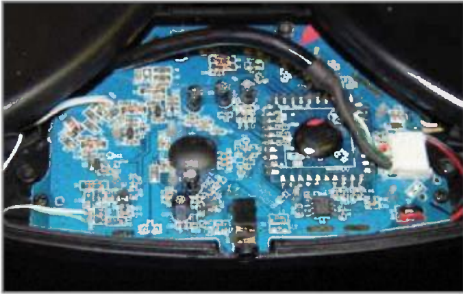
Photo 2 —The drum kit’s PCB is essentially a game controller with some extra triggering circuitry for each drum head. Its fifth input is a bass drum pedal.
