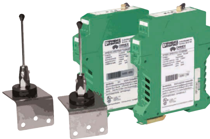
The Phoenix RAD-ICM-900 integrated radio and I/O module eliminates cable and conduit for one 4- to 20-mA current loop and two digital signals in harsh industrial environments.
