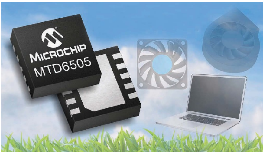
The MTD6505 fan motor driver from Microchip Technology uses a resistor-programmable, sensorless sinusoidal architecture so that you can tailor it to many fan models.
