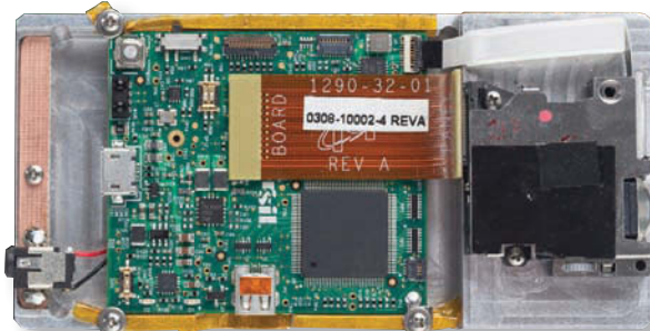
Intersil's Pico-qHD reference design includes an LED driver, a video processor, a power-management IC, a buck-boost converter, and a battery charger.
