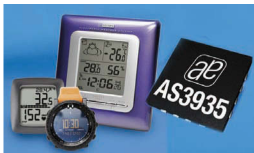
The AS3935 Franklin lightning-sensor IC uses an analog front end and embedded algorithms to sense the approach and proximity of lightning.
