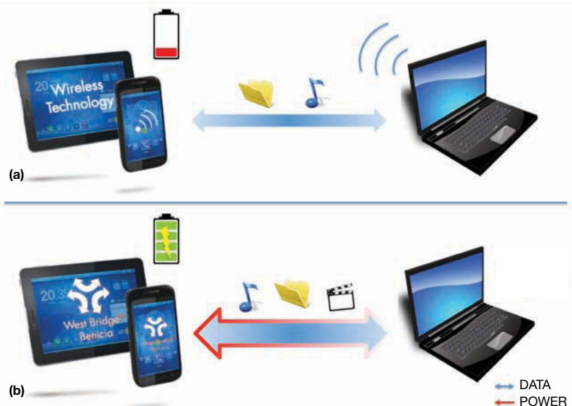
Figure 6 Wirelessly transferring digital content between mobile devices and PCs concurrently drains the device's battery unless it connects to a wall charger or a PC through USB (a). USB 3.0 has versatile connectivity, high bandwidth, and battery-charging capabilities that make it likely to coexist with Wi-Fi on mobile devices for the foreseeable future (b).
