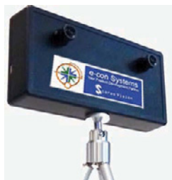
The Capella reference design targets companies that want to integrate stereo vision into their products. It features 3-D analytical applications, such as machine vision.
