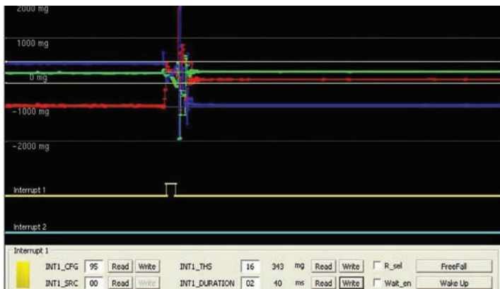
Figure 1 The accelerometer's evaluation board and its Windows demo software capture the device's raw data and the interrupt signal.
