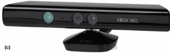
Figure 3 Regardless of the specific 3-D camera technique employed, they all output a depth map of objects they discern (a). A device such as the HTC EVO 3-D smartphone, whose stereo sensor array is primarily intended to capture 3-D still and video images, can also be used for 3-D embedded-vision purposes (b). Microsoft's Kinect (c) harnesses the structured-light method of discerning depth by projecting a known infrared-light pattern in front of it and then analyzing the shape and orientation of the ellipses that it sees (d).
