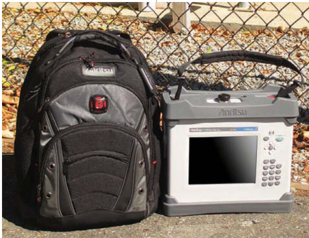
The PIM Master MW82119A runs roughly 2.5 hours between battery recharges.
