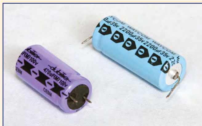
Fig.3. The PCM electrolytic on the left has the negative (-) lead clearly marked, as does the radial lead capacitor on the right. The latter also has an indentation around the body near the positive (+) lead
