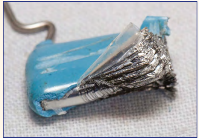
Fig.2. This was a polyester capacitor! It has been cut open to reveal the numerous layers of foil needed to get a value of 100nf into a small volume (it is about 8mm wide)
