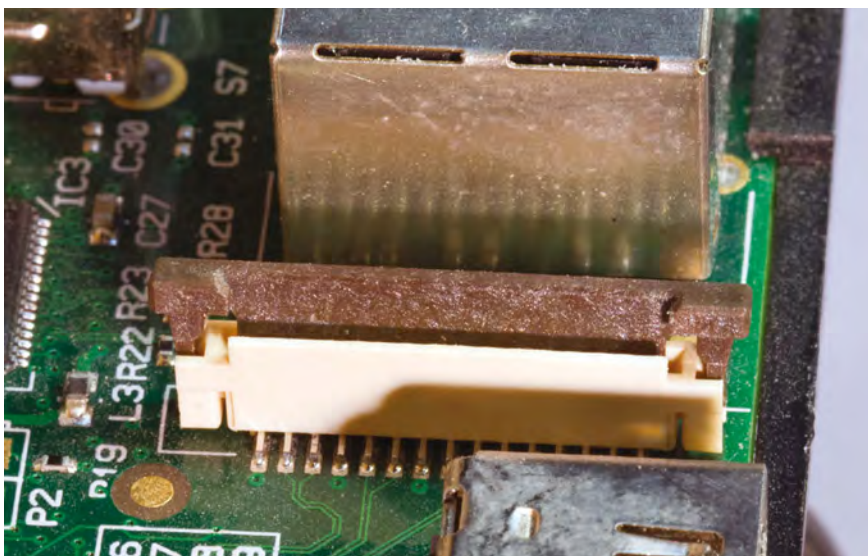
Fig.4. Open the CSI connector by raising the top section slightly. The cable should then fit in quite easily, and the top of the connector can then be pressed down in order to lock the cable in place
