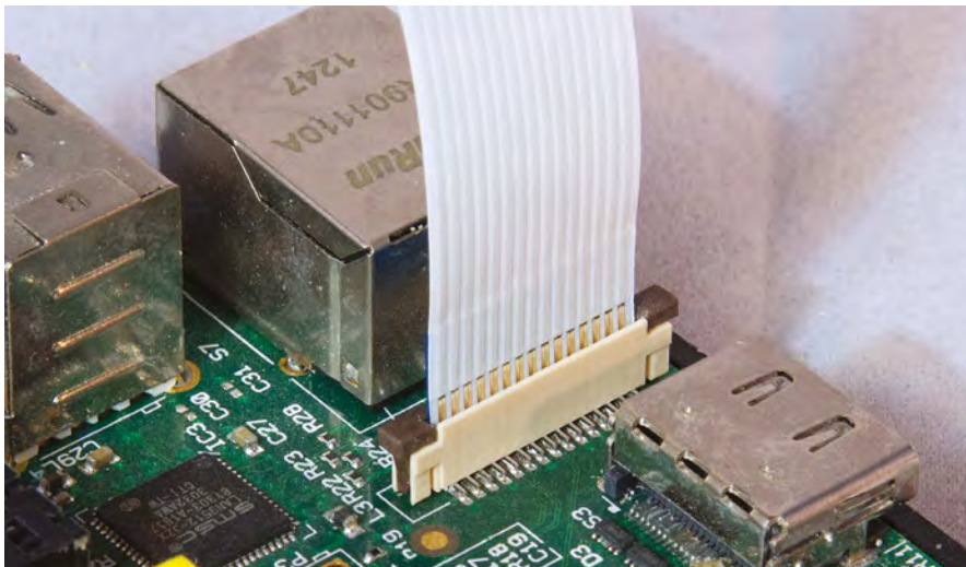
Fig.3. The camera connected to the Raspberry Pi. The cable must be connected to the Raspberry Pi with the plain side towards the Ethernet port, and the silver connectors facing towards the HDMI connector
