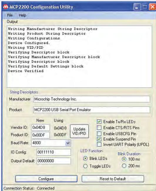
Fig.7: this is the dialog you will see when you launch Microchip's MCP2200 Configuration Utility (except that the Output box will be blank). Configure it as described in the text.
