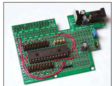
Fig.7.10. Humble Pi prototype 16-channel port expander
