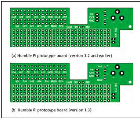
Fig.7.11. Changes to the Humble Pi pin labelling
