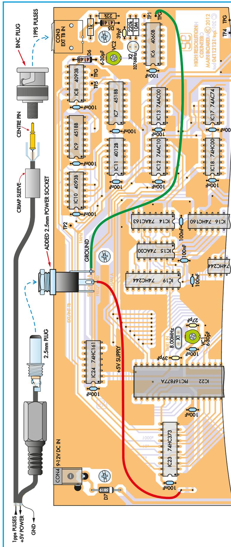
Fig.6: a shielded stereo cable can be used to make the connections between the Deluxe 1pps GPS Timebase and the frequency counter. The 1pps pulses are fed in via the counter's existing BNC socket on the rear panel, while a 2.5mm DC power socket can be added to accept a matching plug to pick up the counter's +5V and GND connections. You can omit this DC socket and the supply connections if you don't intend powering the timebase unit from the counter.
