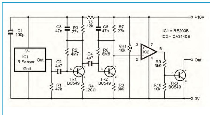
Fig.4. Like the light change detector, this passive infrared detector has a modified output stage that can drive a GPIO input. The light and infrared circuits can be used to drive a single input of the GPIO port, with the two output transistors acting as a simple NOR gate
