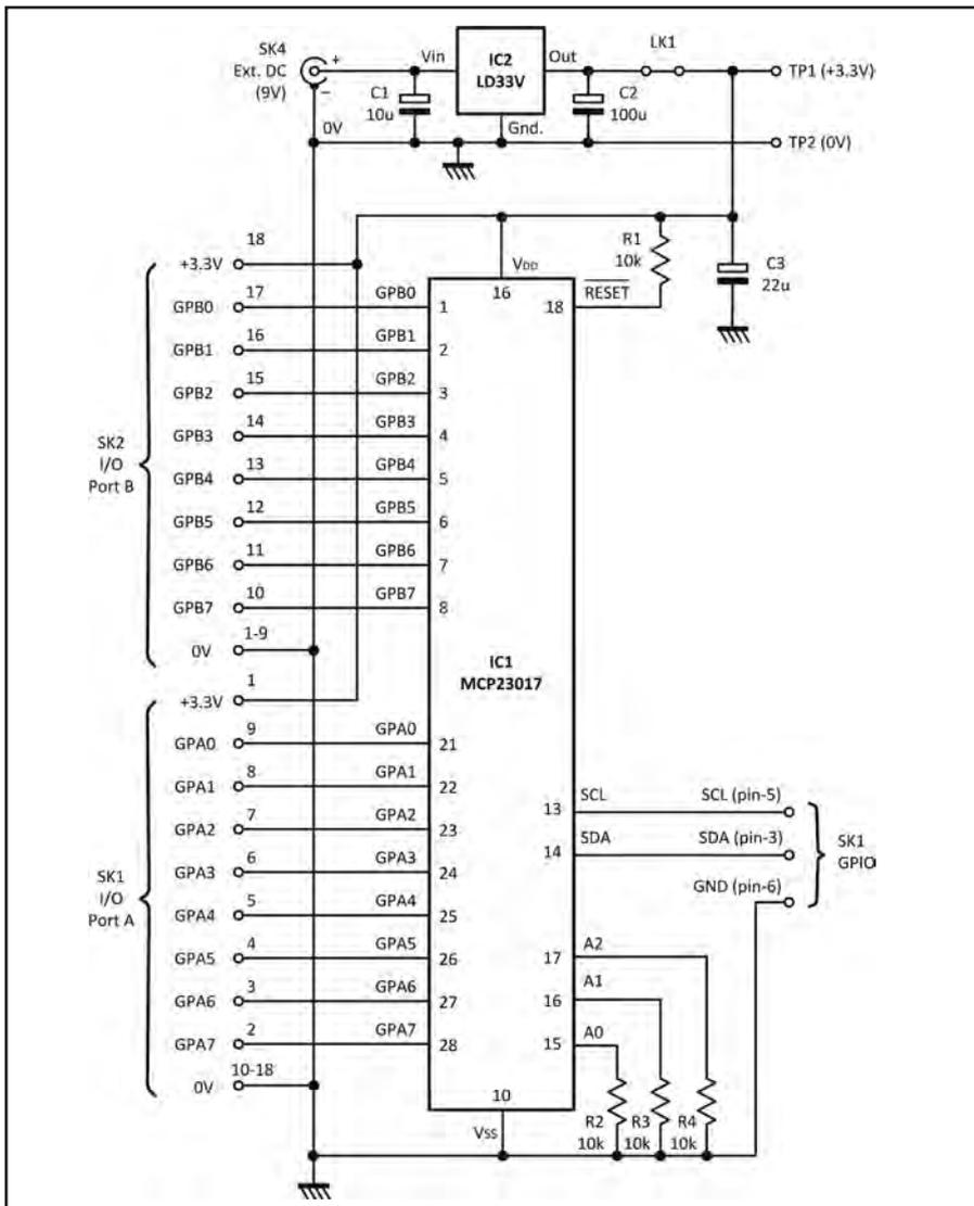
Fig.7.8. Complete circuit of the 16-channel port expander
