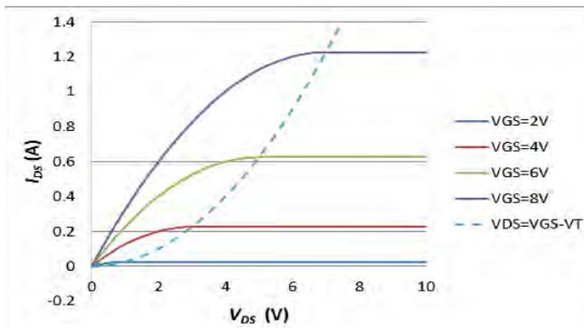
Fig.7. Plot of the MOSFET output characteristics using the appropriate parts of the curves from Fig.3 and Fig.5. The  $V_{DS}=V_{GS}-V_T$  curve (dotted) shows the boundary between the linear and saturated regions of operation
