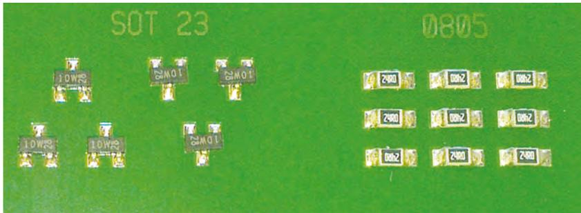
Fig. 12. The board after re-flow (note how the components have re-aligned themselves)
