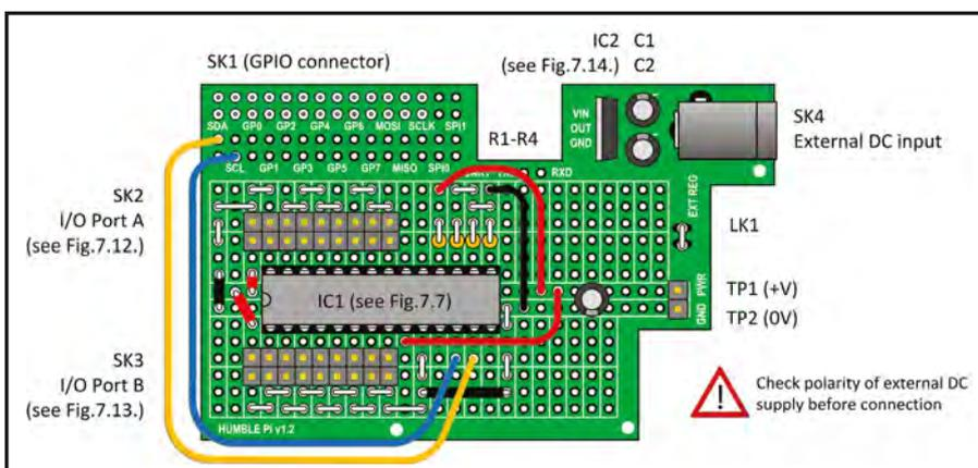
Fig.7.9. Humble Pi prototype board layout
