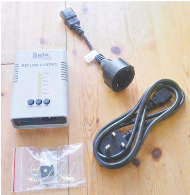
Fig.3. The Oven Controller
