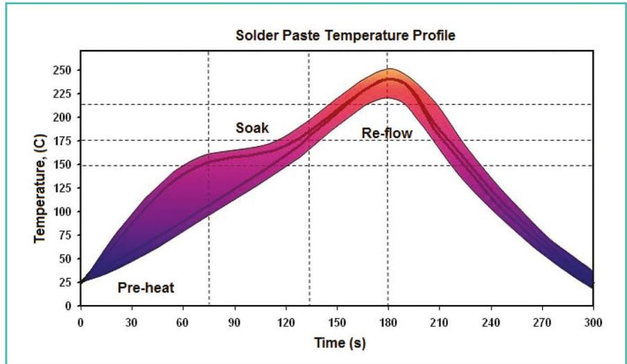
Fig. 1. Solder paste temperature profile
