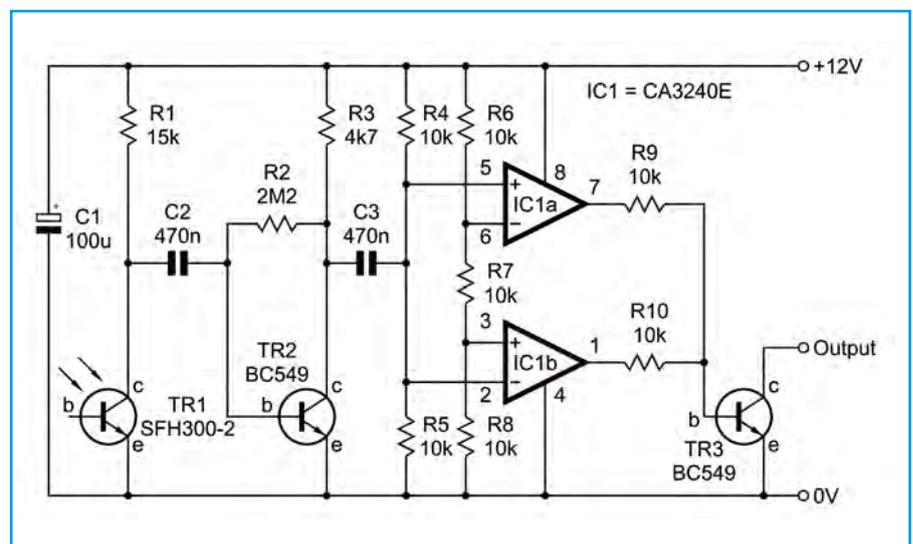
Fig.3. The light change detector circuit. Although it operates from a 12V supply, its open collector output stage can safely drive a 3.3V logic input of the GPIO port
