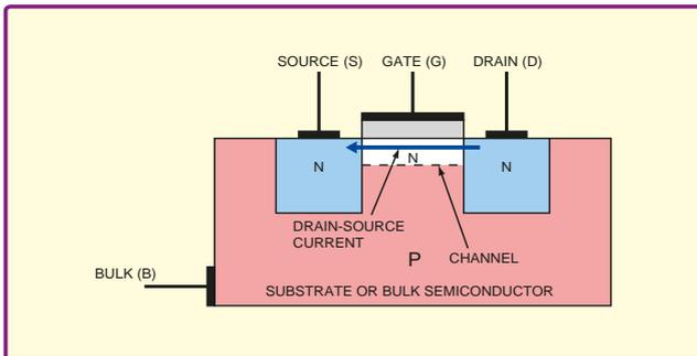
Fig.1. Cross section of N-Channel MOSFET
