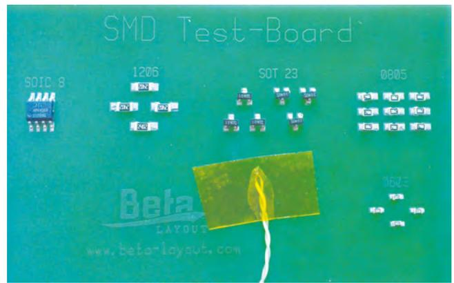
Fig. 11. The board before re-flow (note the badly positioned components)
