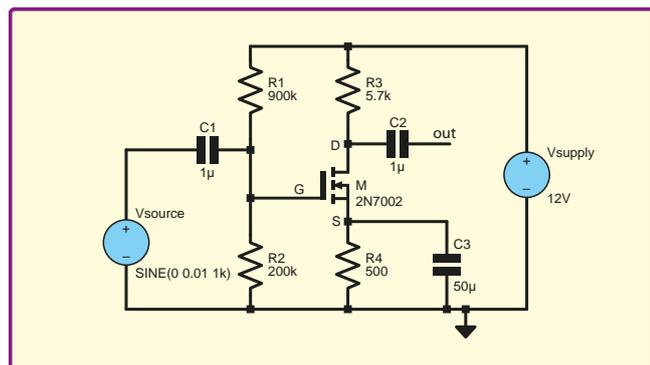
Fig.14. Basic MOSFET amplifier circuit (for LTSpice Simulation)
