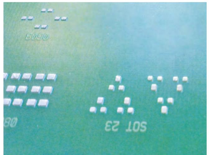
Fig.9. Solder paste on the PCB
