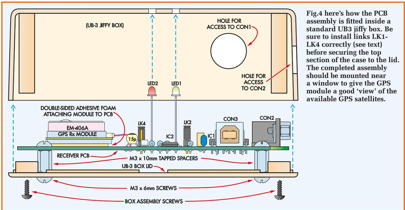
Fig.4 here's how the PCB assembly is fitted inside a standard UB3 jiffy box. Be sure to install links LK1-LK4 correctly (see text) before securing the top section of the case to the lid. The completed assembly should be mounted near a window to give the GPS module a good 'view' of the available GPS satellites.
