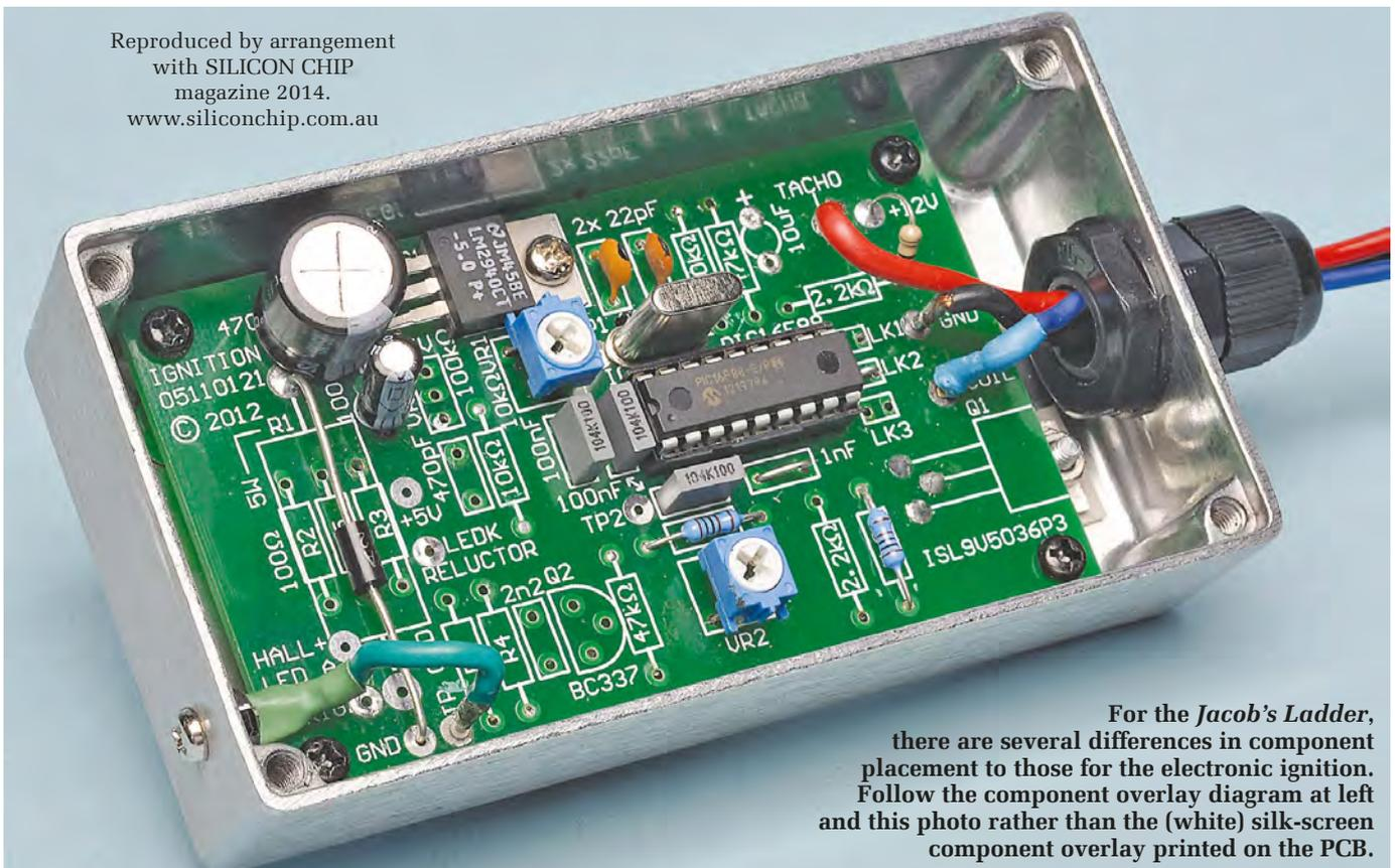
For the *Jacob's Ladder*, there are several differences in component placement to those for the electronic ignition. Follow the component overlay diagram at left and this photo rather than the (white) silk-screen component overlay printed on the PCB.
