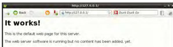
Fig.7.19. Apache test page on the Midori web browser demonstrating a successful installation
