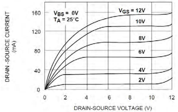
Fig.9. Plot of the MOSFET output characteristics from the ALD1101 datasheet (aldinc.com)
