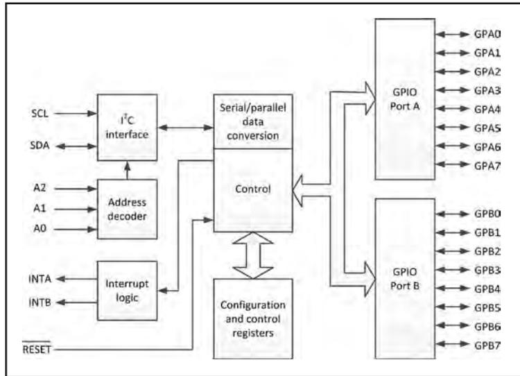
Fig.7.6. Simplified block schematic of the MCP23017 I/O device
