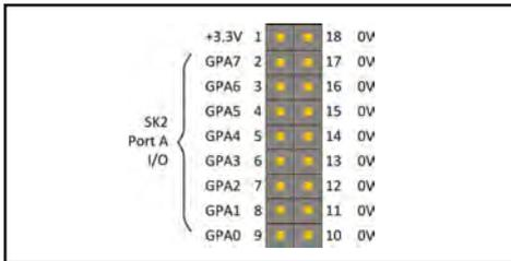
Fig.7.12. Port A I/O connector SK2 pin connections
