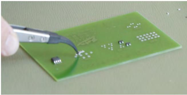
Fig. 10. Placing the components
