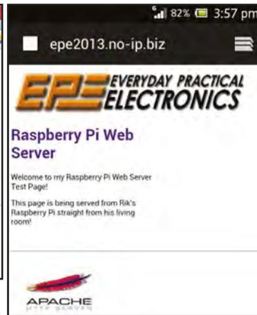
**Fig.7.25. Our test page being viewed on an Android smart phone to test external access**
