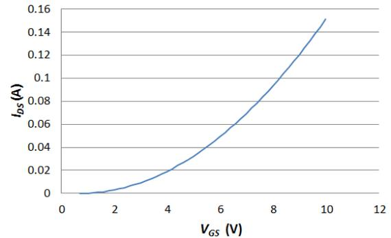
Fig.10. MOSFET transconductance characteristics based on the same equation/data as Fig.5
