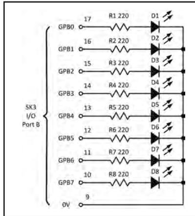
Fig.7.16. LED connection to Port B
