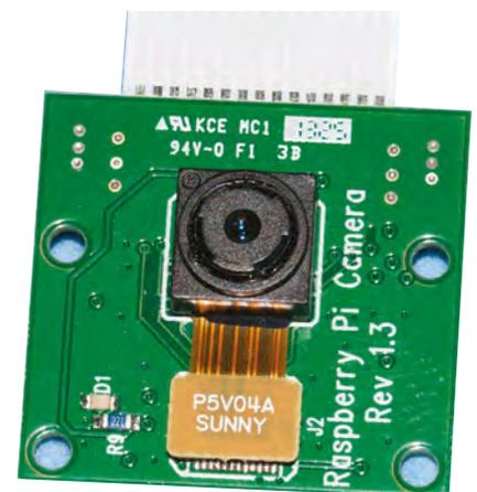
Fig.1. Although tiny, the Raspberry Pi camera module is more sophisticated than one might expect. It has three metering modes and variable ISO sensitivity
