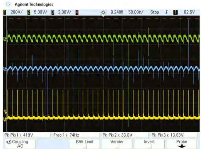
This shows the same waveforms as Scope 1, but with the sweep speed slowed to 50ms/div. This captures more of the spike voltages on the supply lines. Without the input protection components, these spike voltages would be a great deal higher and would damage the regulator. Note that the spike voltages differ because each spark discharge takes a different path across the gap.
