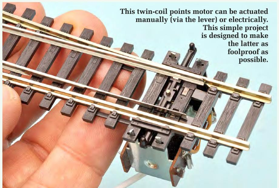
This twin-coil points motor can be actuated manually (via the lever) or electrically. This simple project is designed to make the latter as foolproof as possible.
