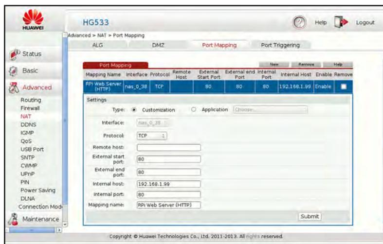
**Fig.7.23. Example port mapping setting screen from a Huawei TalkTalk router**
