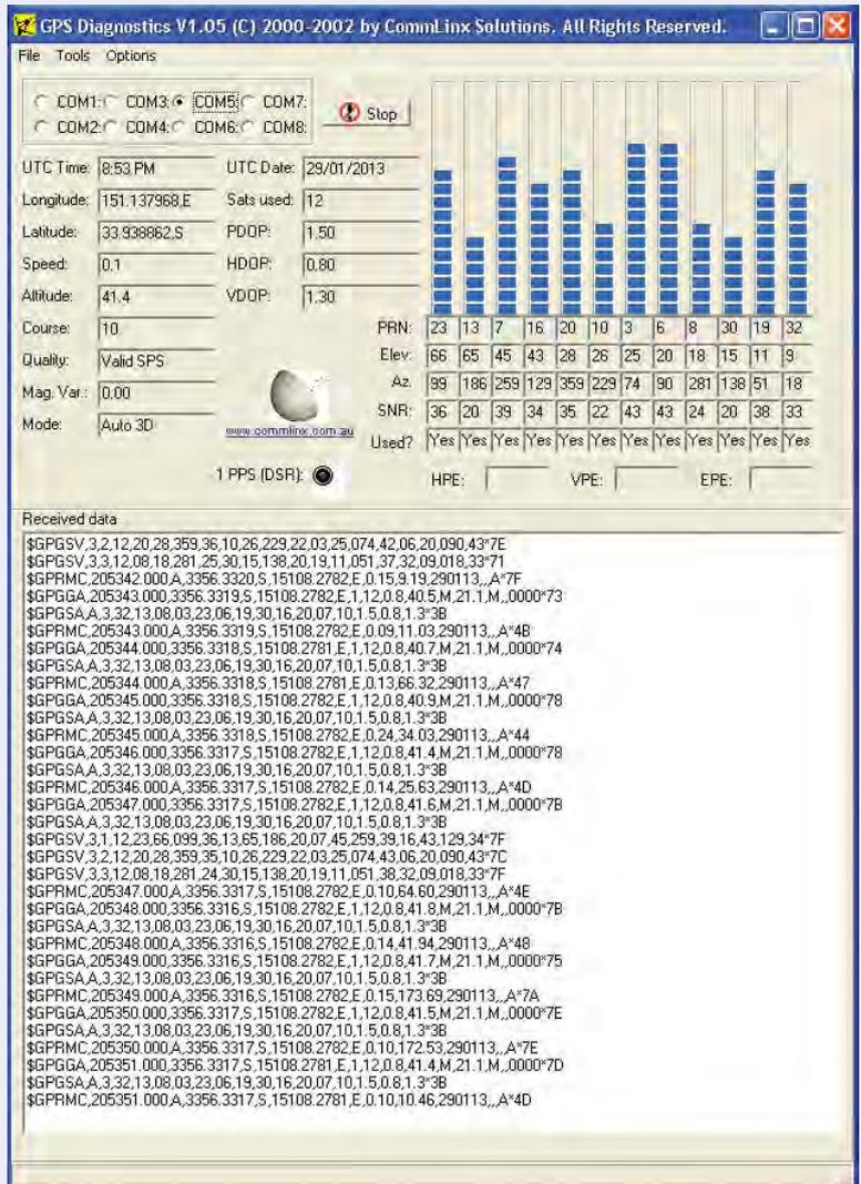
Fig.8: the GPS Diagnostics dialog displays a range of information from the analysed NMEA data, including UTC time, longitude, latitude, altitude, the number of satellites in 'view' and the signal strength from each one.
