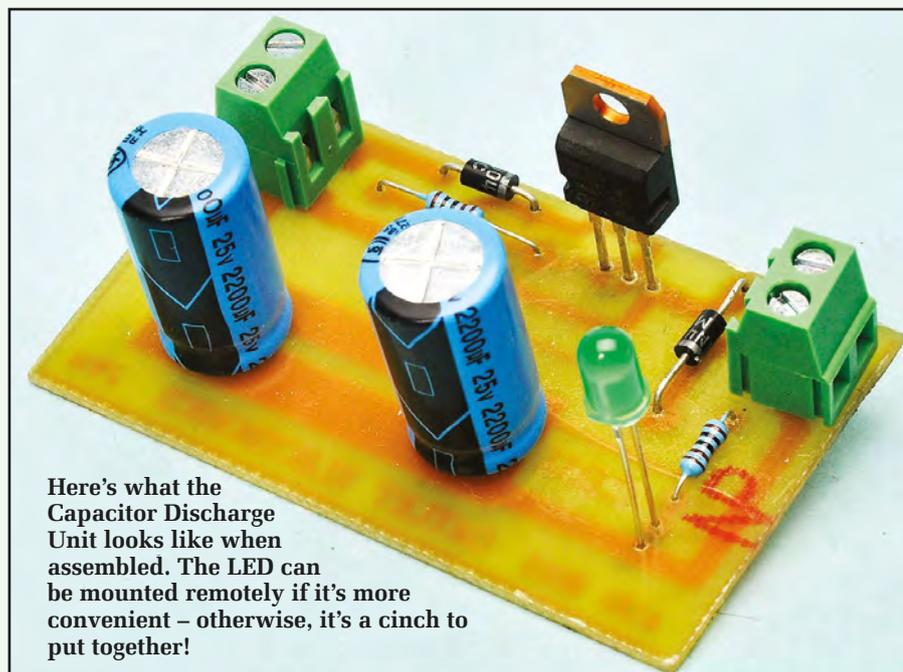
Here's what the Capacitor Discharge Unit looks like when assembled. The LED can be mounted remotely if it's more convenient – otherwise, it's a cinch to put together!
