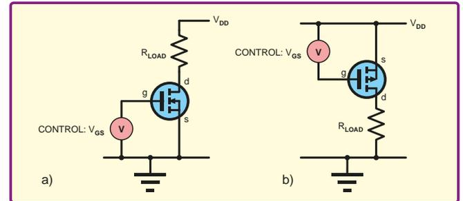
Fig.5. a) N-Channel MOSFET load switching circuit b) P-Channel MOSFET load switching circuit
