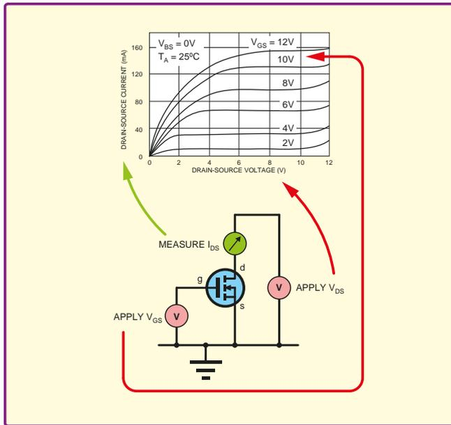
Fig.2. Measuring output characteristics. Note the bulk is connected to the source ( $V_{BS}=0$ ).
