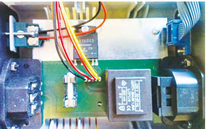
Fig.5. Inside the Oven Controller – power control board
