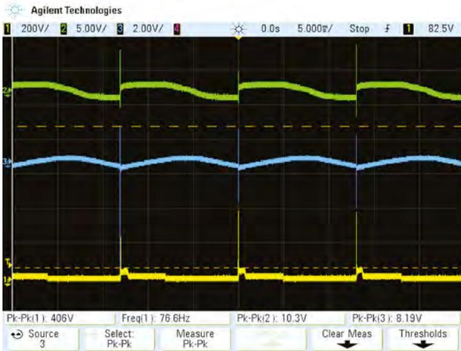
This scope grab shows the *Jacob's Ladder* circuit running at 76 sparks/second and a sweep speed of 5ms/div. The yellow trace shows the high voltages (around 400V peak) at the collector of the IGBT, while the green trace shows the fluctuation on the positive battery rail. The blue trace is the voltage across the transient voltage suppressor (TVS), showing that it is doing its job of protecting the regulator.
