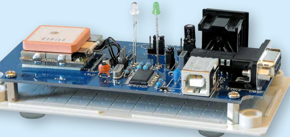
The parts are all installed on a small PCB which is then mounted on the lid of a UB3 jiffy box. The lid then acts as the base of the completed unit shown at left.
