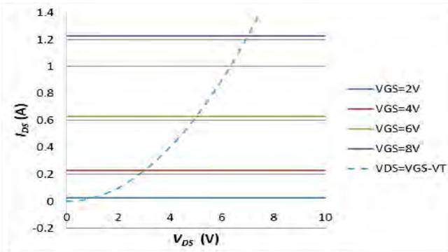
Fig.6. Plot of the MOSFET saturation region equation for various gate voltages. The  $V_{DS}=V_{GS}-V_T$  curve (dotted) indicates the limit of applicability of this equation. It only applies right of this line
