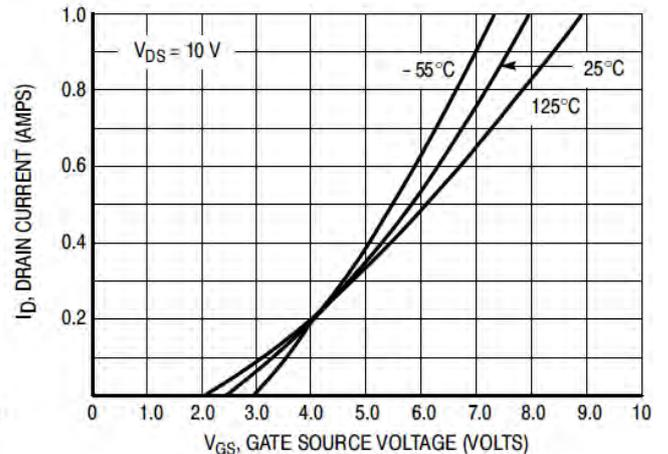
Fig.11. Plot of the MOSFET transconductance characteristics from the 2N7000G datasheet (onsemi.com)
