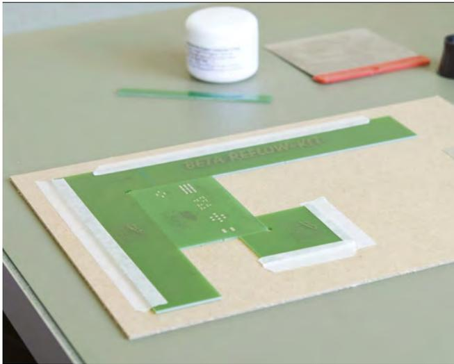
Fig.6. Preparing the PCB 'jig'
