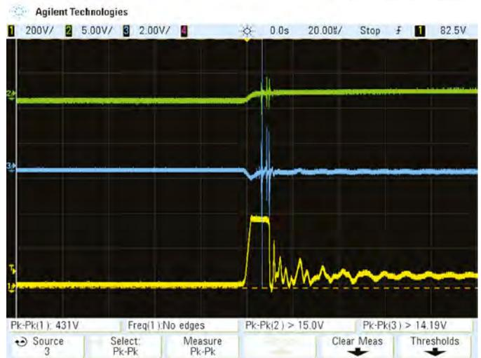
Same conditions as the grab at left, but with sweep speed upped again to 20µs/div. Here we see that the spike voltages across the supply lines are very fast and both are actually clipped by the scope.
