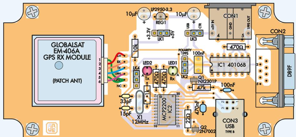
**Fig.2:** follow this layout diagram to build the unit. Omit REG1 and the 10 $\mu$ F capacitor to its left if you are using the Globalsat EM-406A module and install LK1 in the +5V position. Alternatively, install REG1 and the capacitor if your GPS module requires a 3.3V supply and fit LK1 to the +3.3V position.
