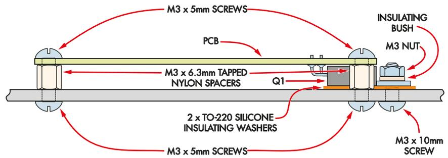
Fig.3: here's how the IGBT is mounted underneath the PCB. 6.3mm nylon spacers hold the PCB at the right height and also insulate it from the case. Two silicone insulating washers are used to insulate the IGBT from the case.
