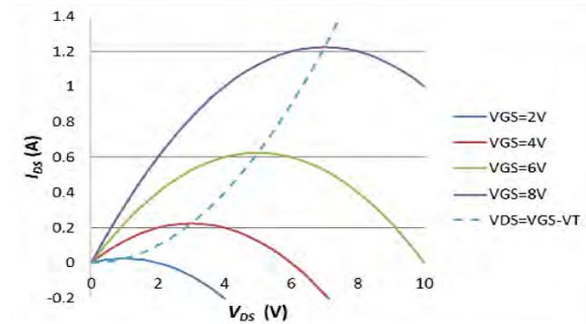
Fig.3. Plot of the MOSFET linear region equation for various gate voltages. The  $V_{DS}=V_{GS}-V_T$  curve (dotted) indicates the limit of applicability of this equation. It only applies left of this line
