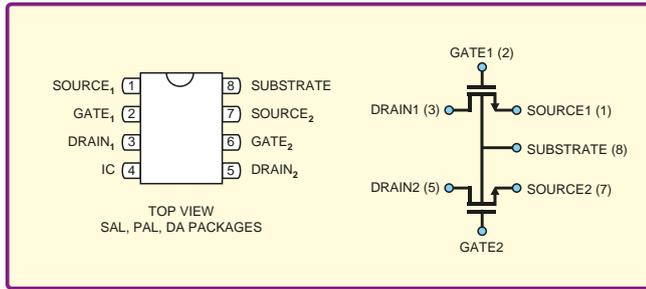
Fig.13. ALD1101 pinout details showing separate bulk connection (aldinc.com)
