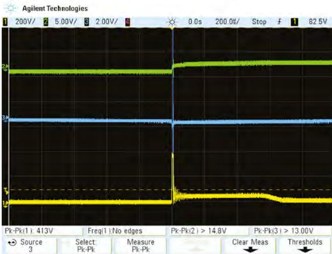
Again, same waveforms as before, but with sweep speed upped to 200µs/div. Here you can see the ringing of the coil primary after the main spike. The voltage is clipped to 413V by the protection limiting inside the IGBT.
