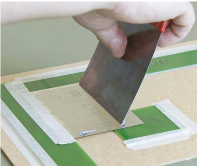
Fig.8. Applying the solder
