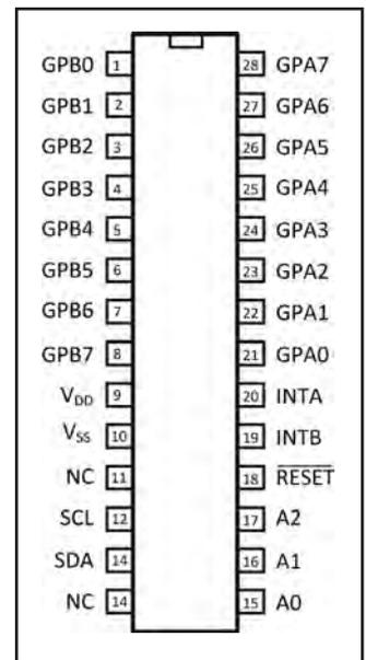
Fig.7.7. Pin connections for the MCP23017
