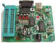
USB/Serial connection. Header cable for ICSP. Free Windows XP software. See website for PICs supported. ZIF Socket and USB lead extra. 18Vdc.
