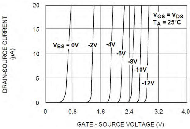
Fig.12. Plot of the MOSFET transconductance characteristics from the ALD1101 datasheet (aldinc.com)
