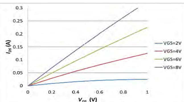
Fig.4. Plot of the MOSFET linear region equation for small values of  $V_{DS}$ . Note the (almost) straight-line relationship between voltage and current indicating a resistor-like behaviour
