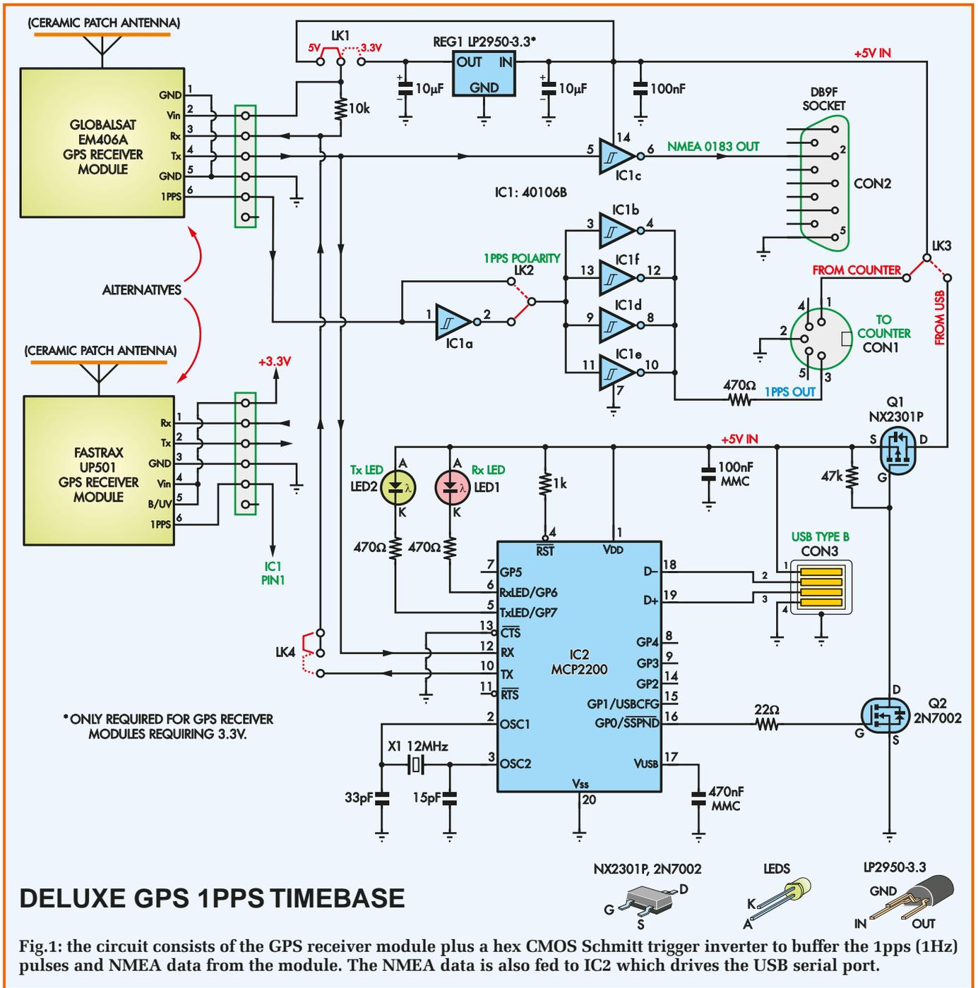
As with the no-frills circuit, link LK2 is used to allow the 1pps pulses to be either inverted or not by the buffer, so that their leading edges are positive-going regardless of their polarity out of the GPS module (some modules may output them as inverted).
