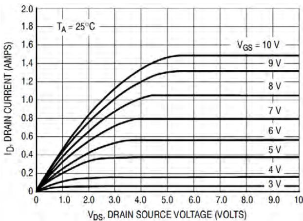
Fig.8. Plot of the MOSFET output characteristics from the 2N7000G datasheet (onsemi.com)
