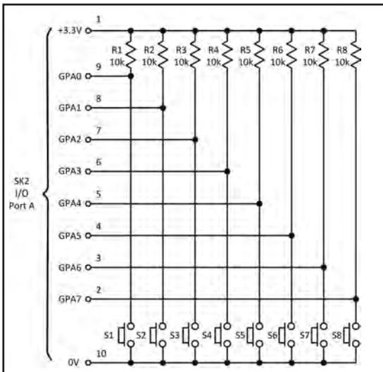
Fig.7.17. Switch input connections to Port A
