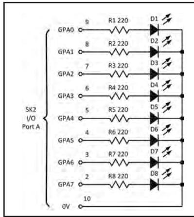
Fig.7.15. LED connection to Port A
