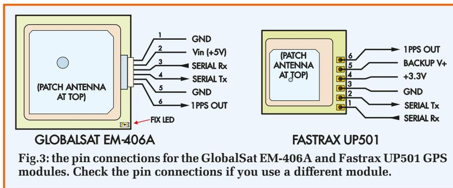
secured to the top of the PCB using a 25mm-square piece of double-sided adhesive foam – see Fig.4. Make sure you attach the module with its patch antenna facing up – it won't work very well if it faces down!
