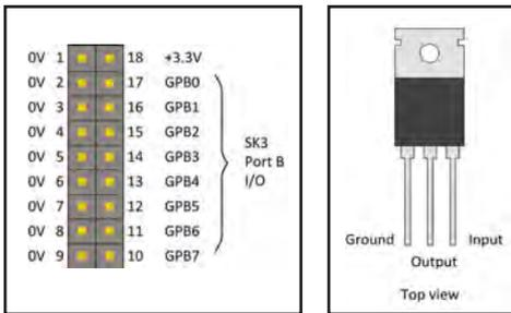
Fig.7.13. Port B I/O connector SK3 pin connections
