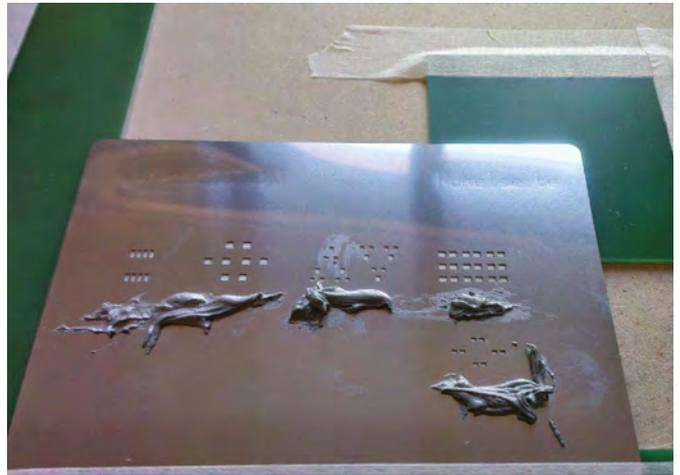
Fig.7. Adding solder to the stencil
