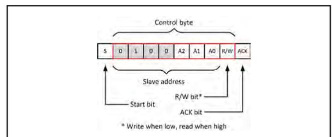
**Fig.7.18. Format of the MCP23017's I<sup>2</sup>C control byte**
