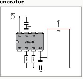
ATtiny13 AM signal generator described here produces short pulses at a frequency of 70 kHz. This results in strong harmonics covering the entire long-wave and medium-wave spectrum. The pulse train is also briefly interrupted at regular intervals to produce amplitude modulation at a frequency of 750 Hz. A radio can therefore receive an AM test signal at 70 kHz, 140 kHz, 210 kHz, etc. and demodulate it to produce a humming tone.
