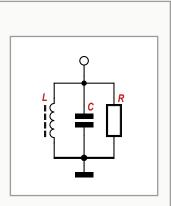
However, in practice the oscillation is damped because energy is dissipated in the form of heat due to the resistance of coil winding, magnetic losses in the core of the inductor, and electromagnetic radiation. For the sake of simplicity all of these losses can be collectively represented by a resistance R in parallel with the circuit. The resonant frequency f is given by the formula:
