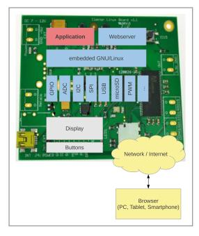
Linux's modular structure makes it the ideal basis for all sorts of projects in measurement and control. A custom control system can be written in virtually any programming language you choose, with the user interface served up as a web page to a PC, tablet or smartphone. In this article we will connect the Elektor Linux board to a typical home network and then show how to write our own server application. We finish with a look at the Lua scripting language.
