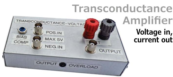
A transconductance amplifier is a special differential amplifier where the output current is a function of the difference in the input voltages. With the help of an AD844, made by Analog Devices, it becomes a simple matter to create such a circuit. A transconductance amplifier like this can be used as a versatile amplifier stage for a wide range of measurement functions, as you'll see in this article.
