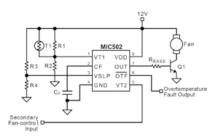
Figure 2. Application example using the MIC502.
