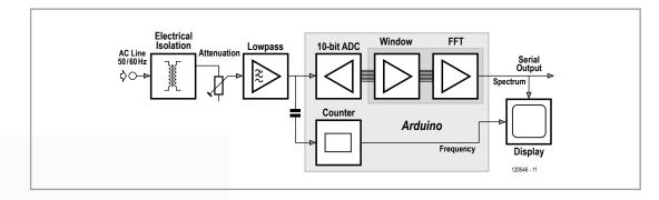
Figure 1. Block diagram for the spectrum analyser.
