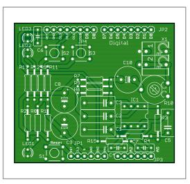
Figure 3. The PCB layout for the filter shield.
