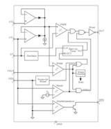
Figure 1. Block diagram of the MIC502.
