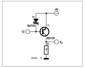
ment circuit for an NPN transistor is shown in Figure 6. The -5 V power supply at the emitter makes it possible to connect the measurement resistor (R1) to ground. The voltage across this resistor  $(1 \ \Omega)$  is proportional to the collector current. The TZ connection of the pre-amp is connected to the base of the transistor. The base current is equal to 1 mA/V. Schottky diode D1 protects T1
