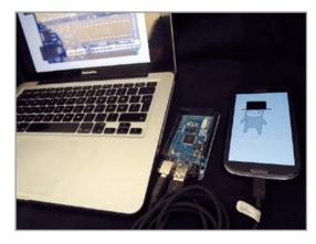
Figure 1. Arduino Mega ADK with Tinker Kit Shield and phone.
