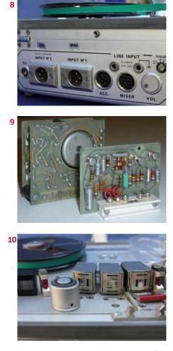
The device was constructed in modular fashion, which was pioneering for the time, with a motherboard on which all modules were arranged. Everything plugged in, using locking gold contacts (**Figure 6**).
