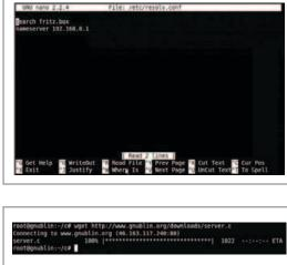
between the board and the internet, we can directly download some example source code for a server. The command 'wget', which will be familiar to users of Linux on PCs, lets us transfer any file we like from the internet onto our board.
