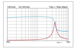
Figure 5. An impedance measurement of an inductor, made with
