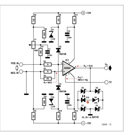
from Figure 1. On TZ you can connect any type of component (also semi-conductors) or a network. Since there is no feedback there aren't any stability issues. The impedance  $Z_{TZ}$  does introduce a measurement error, but the value of this is very small in most applications. The voltage at TZ ( $V_0$ ) is made available via buffer B2.
