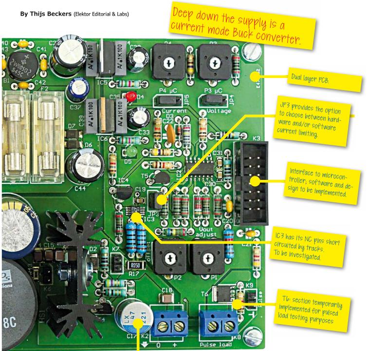
C17 has specs by design, which are only met by a special Nichicon cap. Availability?! ESR measurement results on C17 were unsatisfactory (0.4xx ohms). Measurements conducted 'the old fashioned way' were inconclusive at first. It turned out to be a ground loop between the measurement devices messing up the measurements.
