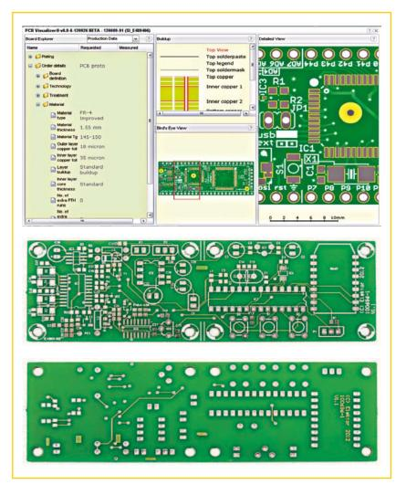
files (Extended Gerber or CadSoft Eagle V6) and conveniently displays a preview of what the PCB will look like after production. Any design error or ordering mistake can be nipped in the bud at this moment, as an extended overview of parameters is displayed on the left, while the board can be viewed in detail on the right.
