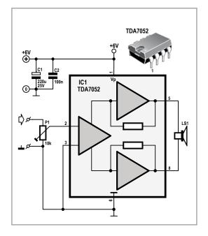
There are countless situations and systems devisable in which a sound signal needs to be amplified in order to drive a (small) loudspeaker, but where space constraints rule out the use of a regular sized amplifier. For these situations, this sub miniature amplifier is perfect. With some skills it can be assembled to a size smaller than an after dinner mint!
