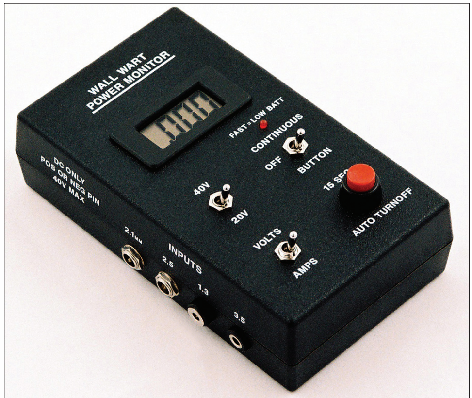
■ FIGURE 2. The new self-contained in-line Wall Wart Power Monitor displays readings either continuously or at the touch of a button.
