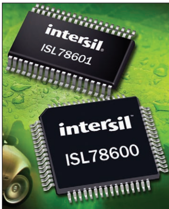
■ Intersil's ISL78600, an automotive-grade Li-Ion battery management system, shown with an ISL78601 battery monitor.
