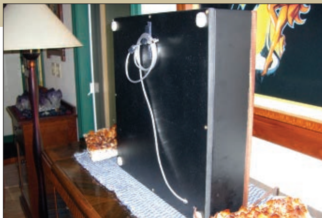
FIGURE 2. PLEASE NOTE: The USB programming cable and power cable protrude from the rear of the portal. I used Velcro® to secure the USB cable when not in use.
