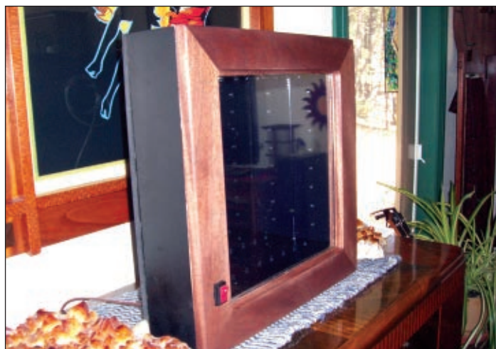
FIGURE 1. My enclosure measures 17" x 17" x 4.75" and is constructed from MDF and walnut wood.
