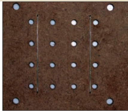
Figure 20. Jig base with two tinned wires loaded.
