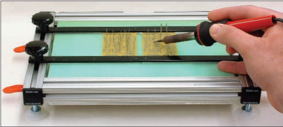
■ FIGURE 8. Jig oriented for soldering. Note leaded components held in place by foam.
