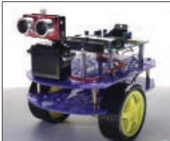
Scooter prototype with RoboProp advanced controller and ultrasonic range sensor head.
