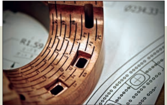
■ Interior portion of the split coil magnet.
