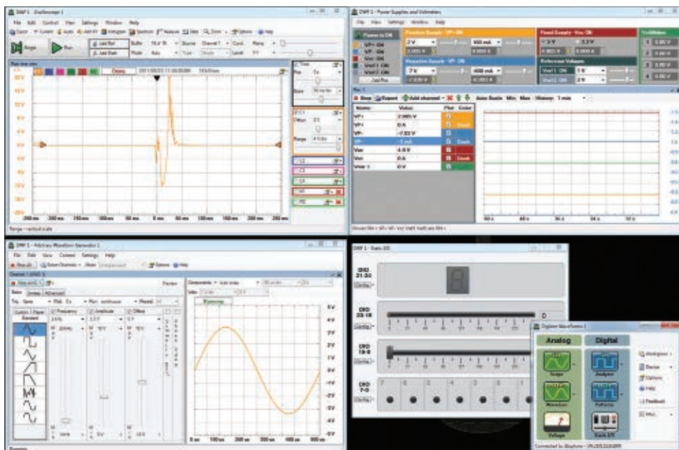
FIGURE 5. Clockwise from top left: Virtual oscilloscope, power supply/voltmeter, waveform generator, and digital I/O configuration panel.
