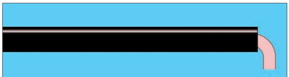
■ FIGURE 4. The end of one of the antenna elements. Leave the rest of the insulation on the wire.
