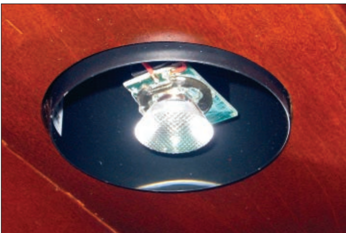
■ FIGURE 6. LED and heatsink assemblies mounted to the incandescent light fixture.
