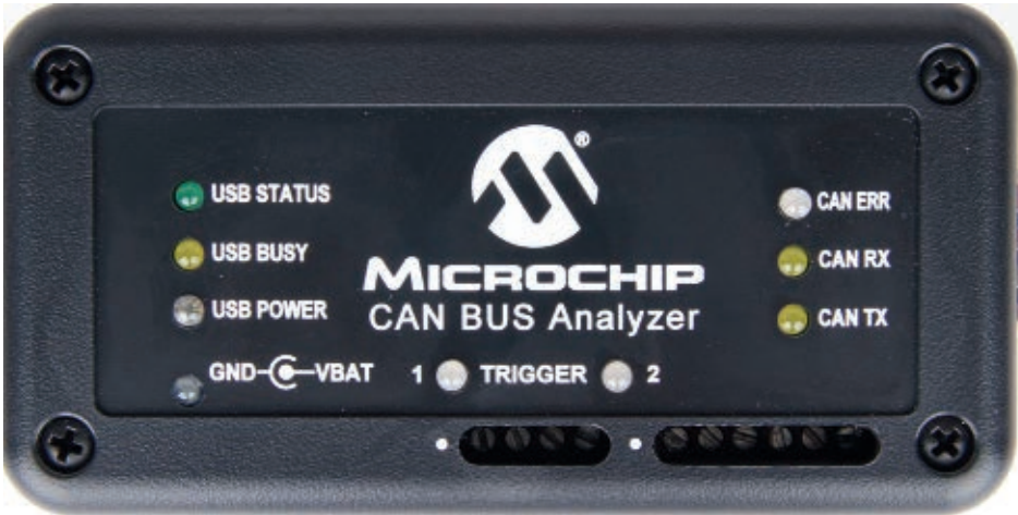
■ PHOTO 2. The Microchip CAN bus analyzer tool is akin to an Ethernet Sniffer. Everything that is thrown onto the CAN bus is captured for your reading entertainment.
