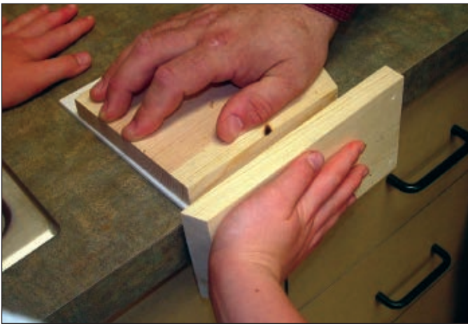
■ FIGURE 13. Syntra can get hot and you probably don't want to leave your finger prints in the warm plastic. Therefore, use a flat board to bend the warm Syntra. Don't use a sheet of metal as it cools the Syntra too quickly.
