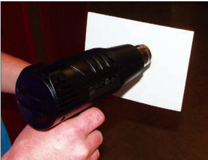
■ FIGURE 12. Keep the hot air gun moving to evenly heat the Syntra, both on top and on the bottom. It's safer if you do this heating where there is adequate ventilation.
