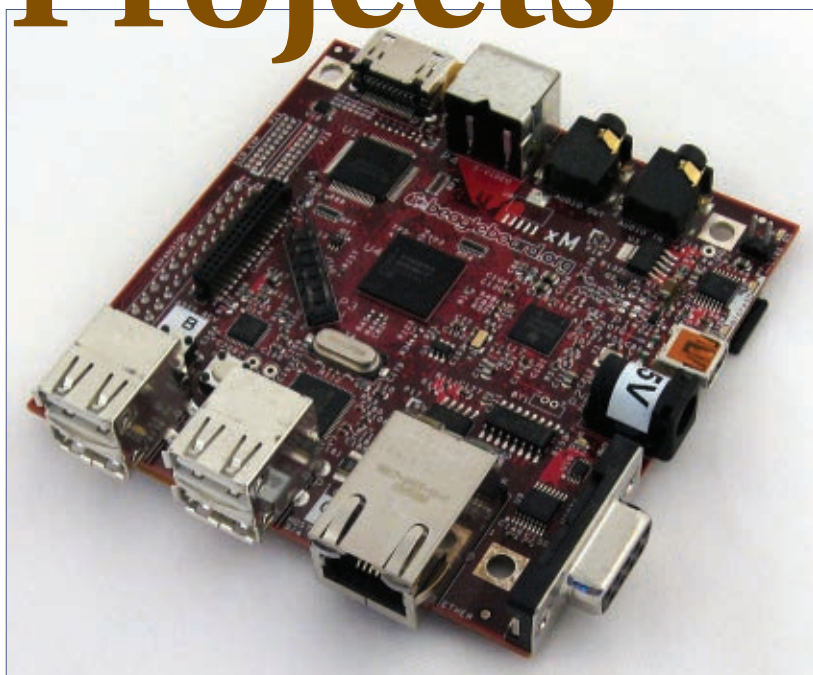
FIGURE 1. The BeagleBoard-xM has four USB host ports and one USB OTG port.
