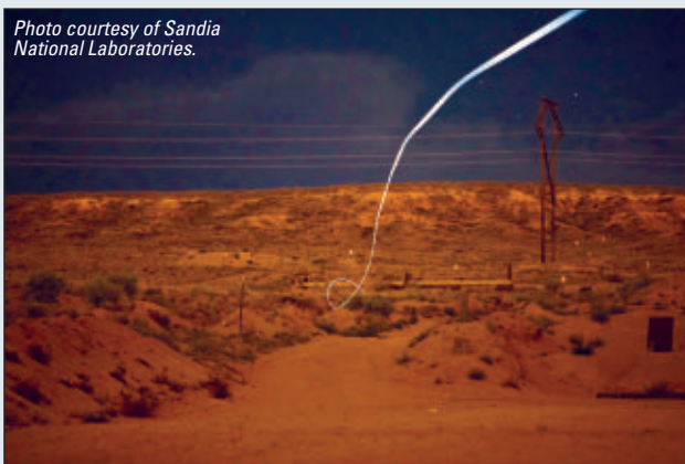
■ An LED attached to a self-guided bullet shows the track to the target.
