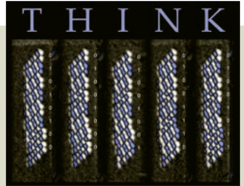
■ A 96 atom magnetic byte imaged in five different magnetic states representing "THINK" in ASCII.
