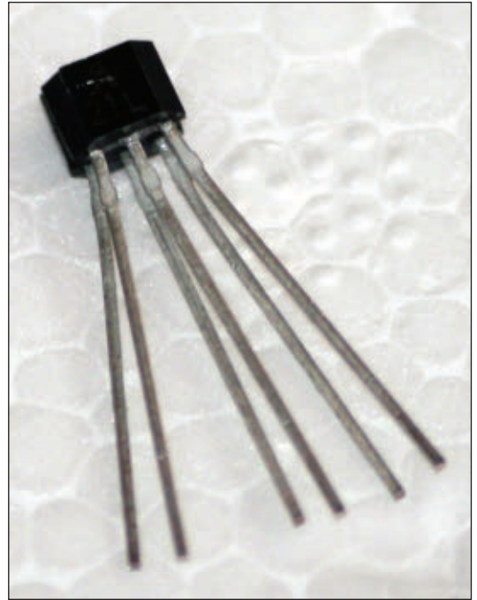
■ FIGURE 2. Since they all have the same orientation, are all powered by the same source, and are very close to one another, they should ideally all read the same. In reality, there are slight chip-to-chip differences. You can just move down the row of chips, recording their actual output voltages and then pick the two that are closest to equal. Once you've found two that match, you glue them back-to-back and get the package shown. (As a side note, you could, in fact, glue them face-to-back so they are facing the same way. If you do this, the difference in signal outputs will now represent the gradient of the magnetic field. Instead of telling you how strong the field is, it will tell you how much it changes over that tiny distance of a millimeter or two. If you decide to build one of these, you might want to put a spacer between the two chips so they are a centimeter or so apart.)
