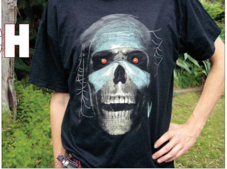
■ FIGURE 1. This interactive Halloween spook shirt uses an Arduino and an Adafruit Wave Shield to add lights and sounds.
