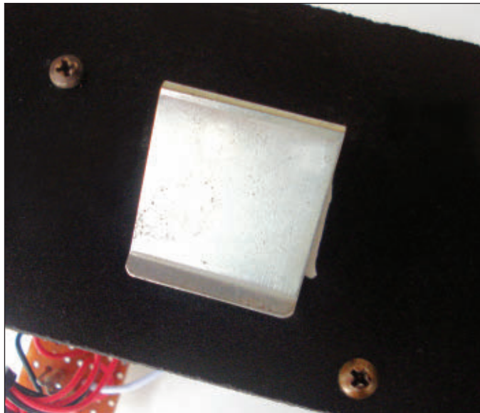
■ FIGURE 9. Use a nine volt battery holder as a belt clip on the back side of the plastic base.
