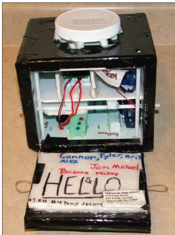
■ FIGURE 2. This is one of the student BalloonSats. It's a six inch cube with a temperature and relative humidity sensor on top (under the plastic lid) and a digital camera looking out the right side.
