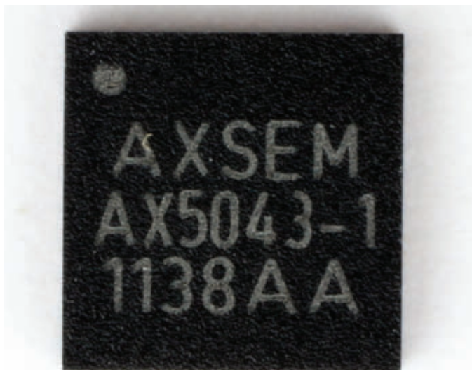
■ PHOTO 1. The AX5043 is a narrow-band ultra-low power RF transceiver IC. This RF IC can be programmed to operate with a carrier frequency range of 70 to 1,050 MHz.
