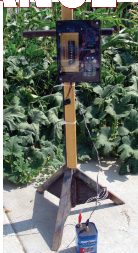
■ FIGURE 1. Finished data logger and camera for remote monitoring using an inexpensive "no contract" cell phone.
