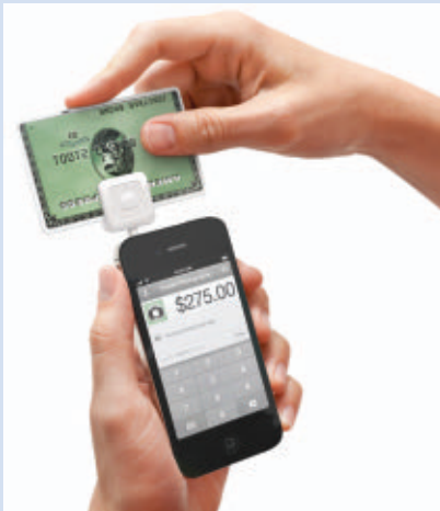
■ FIGURE 2. Square's card reader dongle that turns a smartphone or tablet into a credit card terminal.
