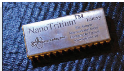
■ The NanoTritium battery provides a 20+ year operating life.
