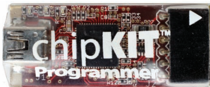
■ PHOTO 3. The chipKIT programmer/debugger is designed to work with the chipKIT Max32, Uno32, uC32, and MX3cK. I've also used it to develop home-brewed PIC designs.
