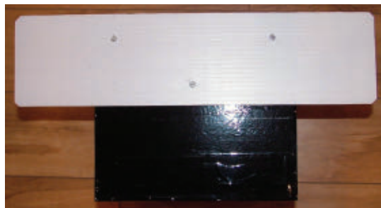
Figure 6: A view from the back. The antenna plane and antenna itself are lightweight; therefore, only three bolts are required to attach the Coroplast plane to the airframe. All bolts in the airframe need to use nylon locking nuts, or nylocks. Their nylon inserts insure they will not rattle loose during a mission.
