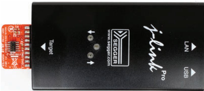
■ Photo 2. In addition to its standard programming/debugging duties, the J-Link PRO's Ethernet interface allows multiple unit debugging over an Ethernet network. Our immediate need is the J-Link PRO's ability to interface to our STM32F030R8T6 using an SWD programming interface. The target socket is loaded with a 1.27 mm SWD adapter.
