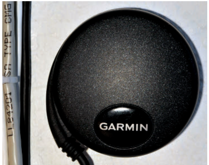
■ FIGURE 6. Using a GPS receiver to extract the time and date doesn't require setting, but an RTC could be substituted.
