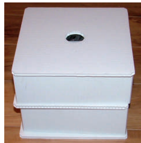
Figure 3: Three pallets and two spacers stacked together created this three level avionics deck. I drilled holes through the center of each pallet after finding out that they were difficult to remove from the airframe without them.
