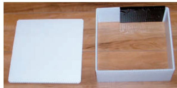
Figure 2: The pallet is a 10 inch square of 1/4" Coroplast and the spacer is made from a sheet of the thinner 3/16" thick Coroplast that was cut, folded, and taped together. Most glue will not adhere to polypropylene, so I resorted to taping the ends of the Coroplast together. The spacer stands four inches tall.
