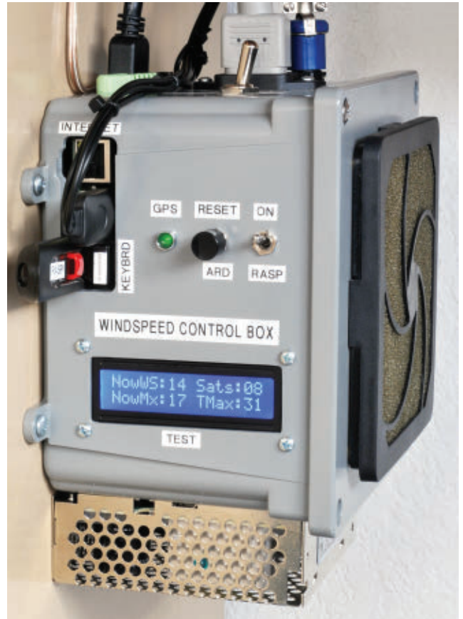
■ FIGURE 4. Here, 8-10 GPS satellites are typically in use (as shown on the LCD), even with the GPS receiver mounted indoors.
