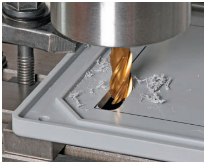
■ FIGURE 7. Fabricating the box and its cover was a snap with my benchtop milling machine. No more filing for hours!
