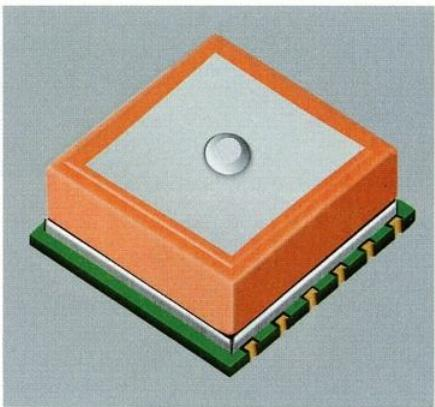
Obr. 4. Modul GPS
