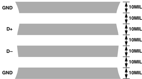
Figure 4. Arrangement of Signal Tracks
