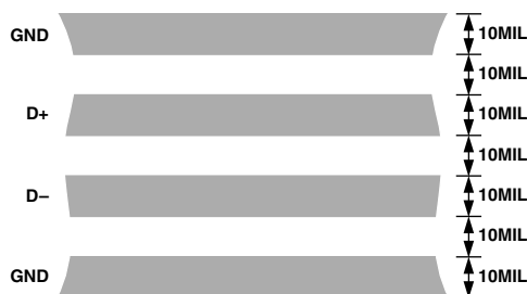
Figure 4. Arrangement of Signal Tracks
