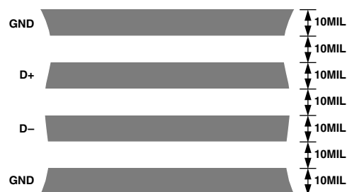
Figure 6. Arrangement of Signal Tracks
