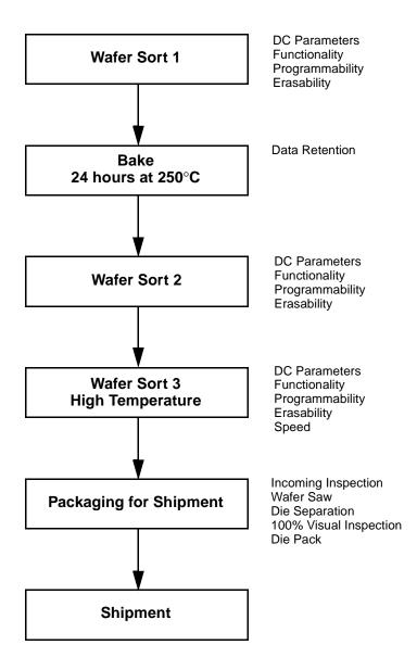
Figure 1. AMD KGD Product Test Flow
