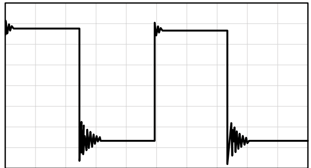
(b) C_L = 130 \text{ pF} , R_L = \text{NO LOAD}
