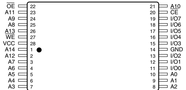
28-Pin TSOP (Standard)
