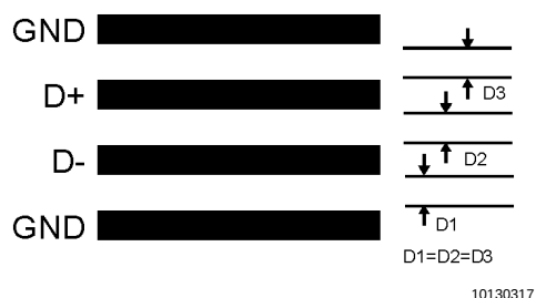
FIGURE 15. Ideal Diode Trace Layout
