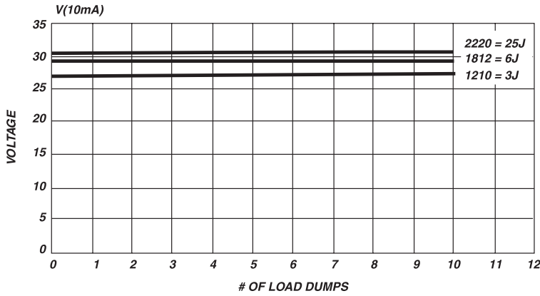
FIGURE 5. AUML LOAD DUMP PULSING OVER A TEMPERATURE RANGE OF -55°C TO 125°C
