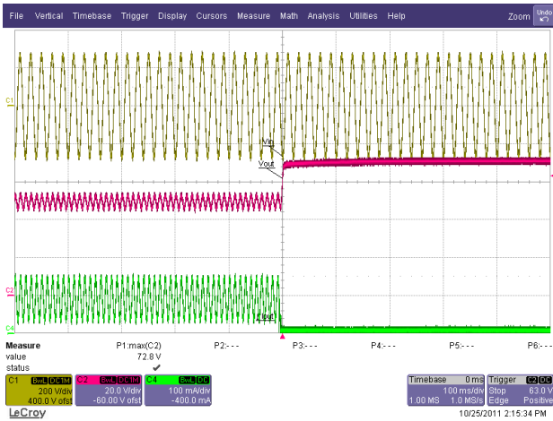
Figure 37 – 190 VAC / 50 Hz, Normal Operation then No-load. Ch1: V_{IN} , 200 V / div. Ch2: V_{OUT} , 20 V / div. Ch4: I_{OUT} , 100 mA / div., 100 ms / div.
