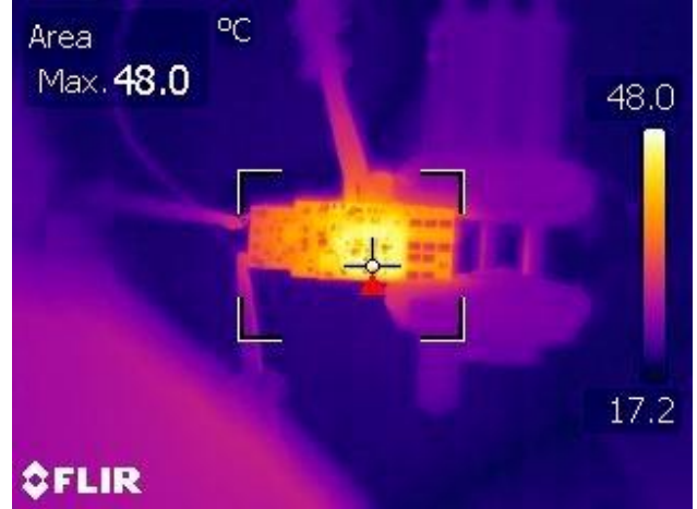
Figure 17 – Bottom Side. R4- Current Sense Resistor: 48 °C.
