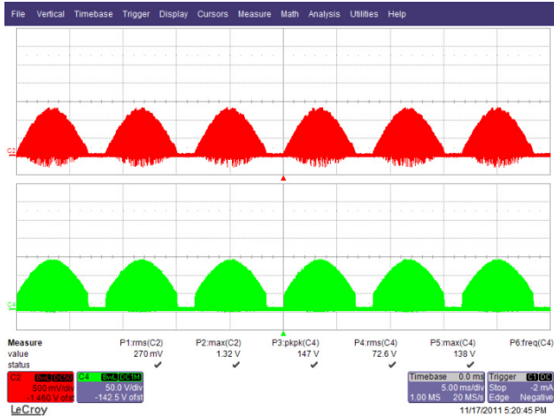
Figure 39 – 90 VAC, 60 Hz. Upper: I_{DRAIN} , 500 mA / div. Lower: V_{DRAIN} , 50 V, 5 ms / div.
