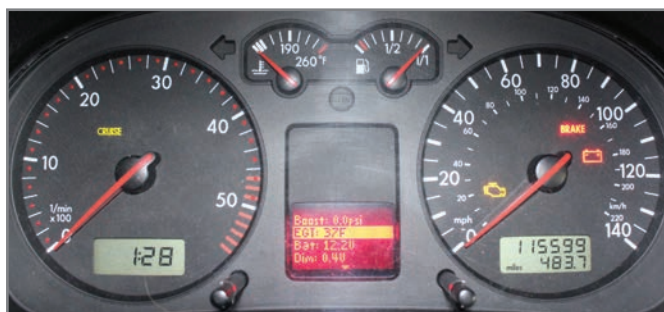
Photo 1 —The original inspiration for the menU system was a microprocessor-based sensor system that I designed and installed in my Jetta TDI. In particular, I needed a way to display and control a variety of different sensors using a small screen mounted between the gauges and the three buttons at the end of the windshield wiper stalk.
