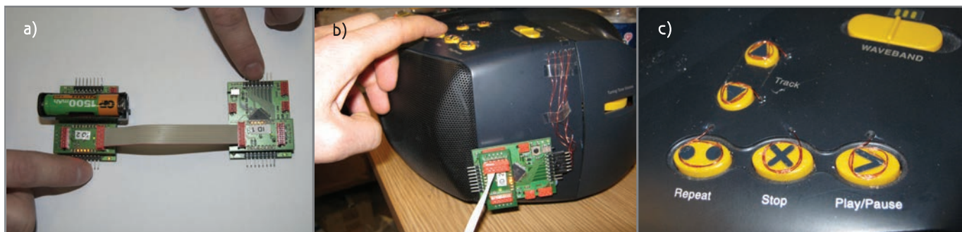
Photo 1a —Two daisy-chained Microchip Technology mTouch boards with a battery board providing the power and LED boards showing the channel status. b —A single mTouch board attached to a CD player with an LED board attached. c —This is a close up of the buttons on the CD player. The thin laminated wire connects to the mTouch board and triggers the detector when touched.
