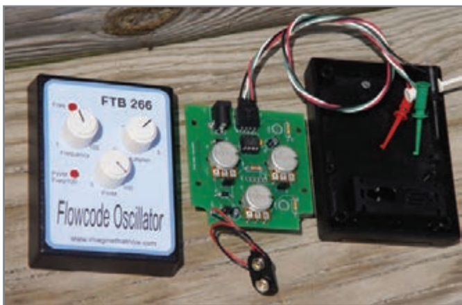
Photo 4 —The PCB fabricated for this project was designed to fit a Pactec enclosure that comes with a 9-V battery compartment. The pots and LEDs are mounted so they will be available from the PCB's solder side. An external cable includes frequency and PWM outputs as well as ground and 5 V.
