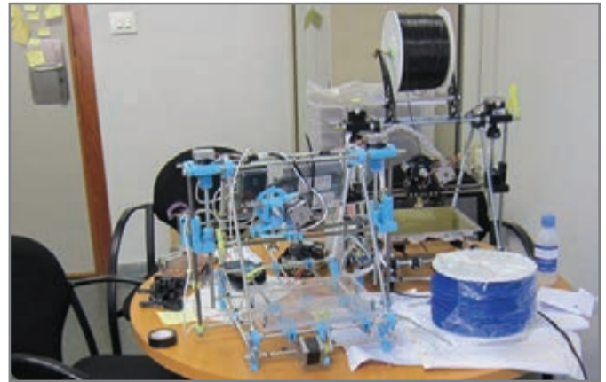
Miguel built two 3-D printers that use plastic filaments. The black one printed the blue parts he used for the second one.
