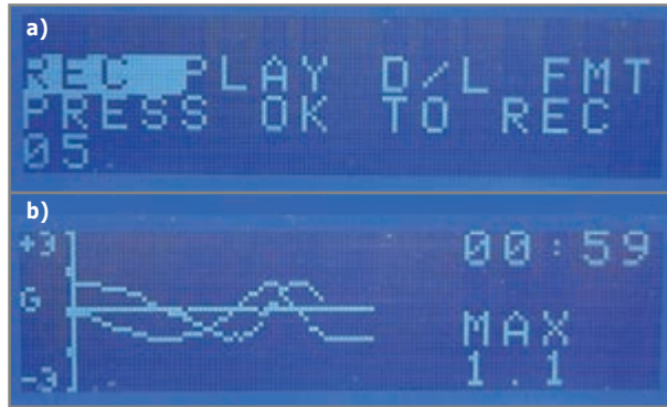
Photo 3 —These are the main menu and record screens, as seen on the LCD. a —The main menu displays four items. The Record function highlighted. When that item was selected with the OK button, the next available memory slot (05) was selected. b —During recording, acceleration data is displayed on a graph along with the maximum value achieved and the elapsed recording time.
