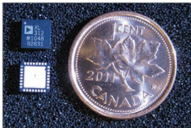
Photo 2 —Look how an Analog Devices ADXL312 digital accelerometer measures up to a Canadian penny. The tiny lead-frame package measures only 5 mm on each side.
