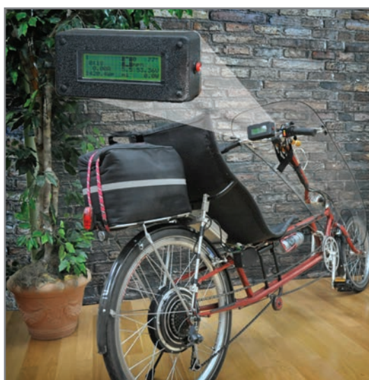
Photo 1 —The EBikeMeter is mounted on an electric-assisted recumbent bicycle's handlebar.
