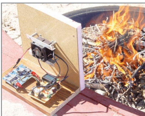
Photo 2 —The project circuitry is mounted behind the insulated surface, which will keep the fire's radiation from cooking the components. The heat-collection sink is facing the fire I've built in a portable fire pit.
