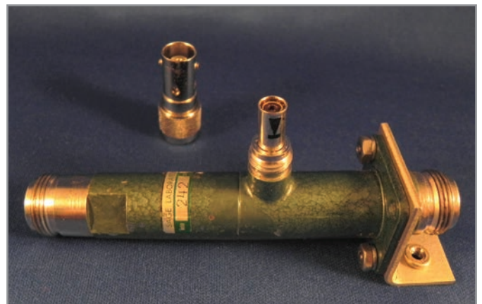
Photo 1 —This is an example of a single-diode mixer, extracted—if I remember correctly—from a 1965 HP8551 spectrum analyzer. The diode is the small cartridge. It is encapsulated inside the BNC connector, which is visible on the back.
