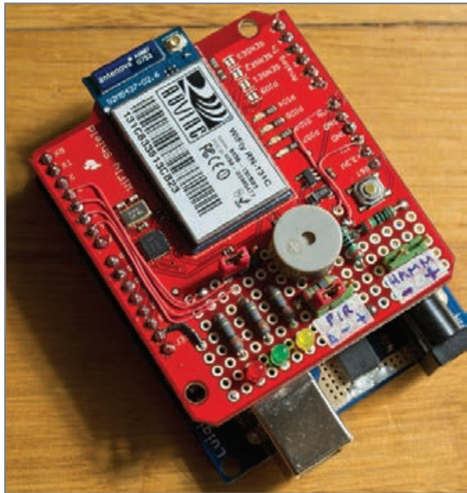
Using a Wifly shield to connect an Arduino to the 'Net
