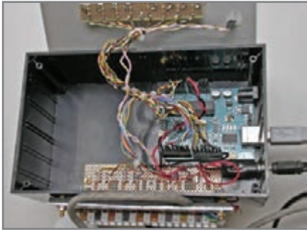
An interface between PIR sensors and an Isadora program
