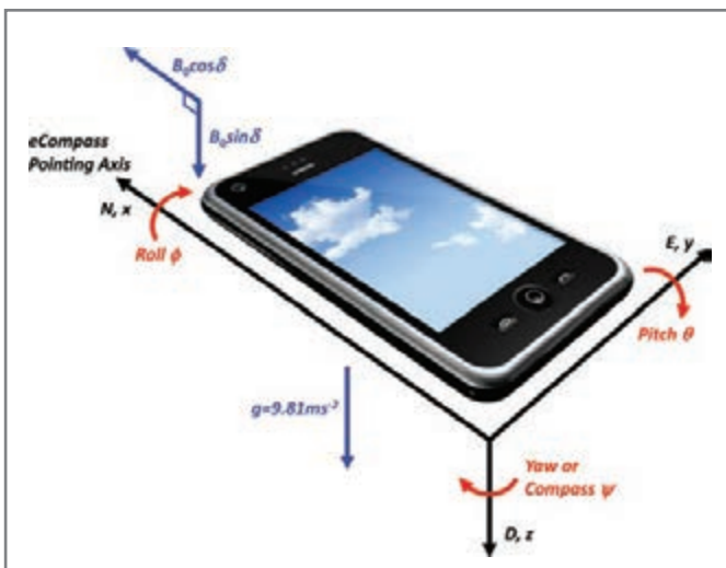
Photo 1—The aerospace north-east-down coordinate system
