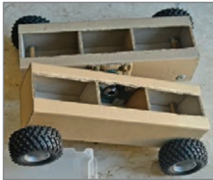
A mockup of the Lino made with corrugated paper to test the validity of the project
