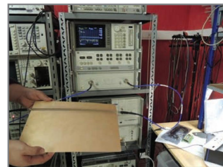
Photo 1 —I use this microstrip transmission line for my experiments. The line is simply a copper track on top of a plain copper ground plane. On the top side, there are still two ground planes on both sides, but they are significantly far from the transmission line. On the back you can see the HP8510 vector network analyzer used to check the setup.
