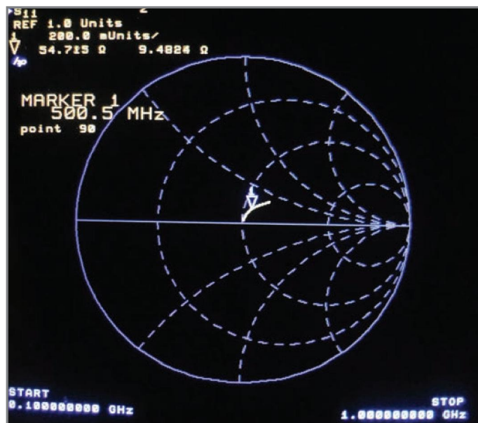
Photo 4 —The 50- \Omega test load was measured on a HP8510C vector network analyzer. On such a plot, a 50- \Omega perfect impedance is at the center. Here the cursor position, at 500 MHz, shows that the measured impedance is not exactly 50- \Omega , more precisely it is measured at 54.7 + 9.4j \Omega . Such a complex impedance includes both a magnitude and a phase measurement.
