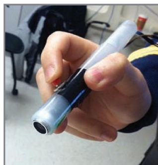
Photo 2 —The pen, which features a mounted push button, was made from an emergency whistle.
