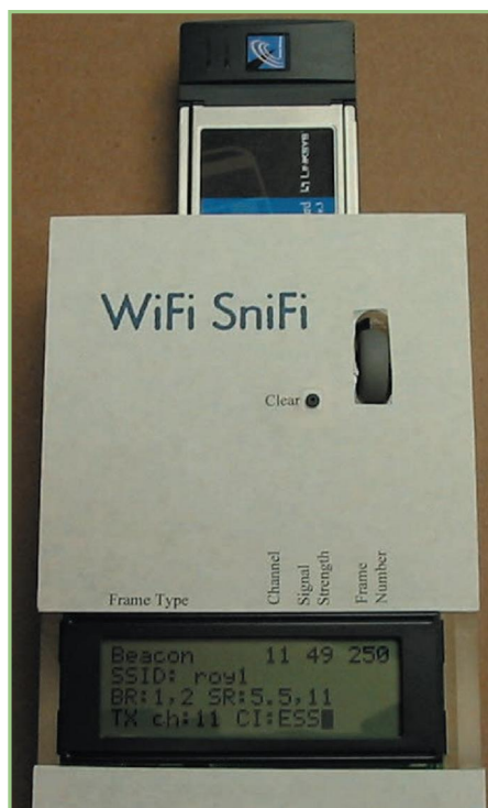
Photo 1 —The WiFi SniFi uses a PCMCIA card to interact with wireless networks, a small LCD to display packet contents, and an old mouse scroll wheel to get user inputs. An 8-bit, 5-MHz microcontroller runs the entire thing.
