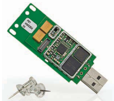
Figure 3 Renesas Mobile Corp has released the SP2531 integrated triple-mode LTE slim modem.
