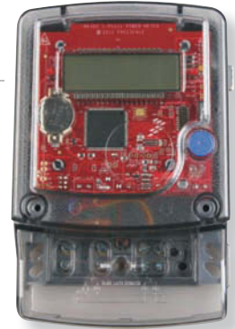
A smart-meter reference design combines Inside Secure’s contactless-NFC-chip technology with Freescale’s secure-microcontroller technology to enable virtually tamperproof secure mechanical meters (courtesy Freescale).
