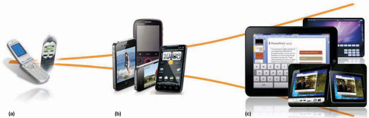
Figure 2 Traffic growth has exploded as manufacturers develop new mobile terminals. In 2000 (a), traffic included 50-kbps GPRS (general-packet-radio service) and RTT (radio-transmission technology). By 2010, with approximately 500 million deployed smartphones, traffic had moved to 5- to 7-Mbps HSPA+ and EVDO (b). By 2020, traffic will move at 1 Gbps (c), with LTE-A, 4 billion new smartphones, 10 billion new smart devices, millions of new apps, and video- and cloud-based services (courtesy 4G Americas).
